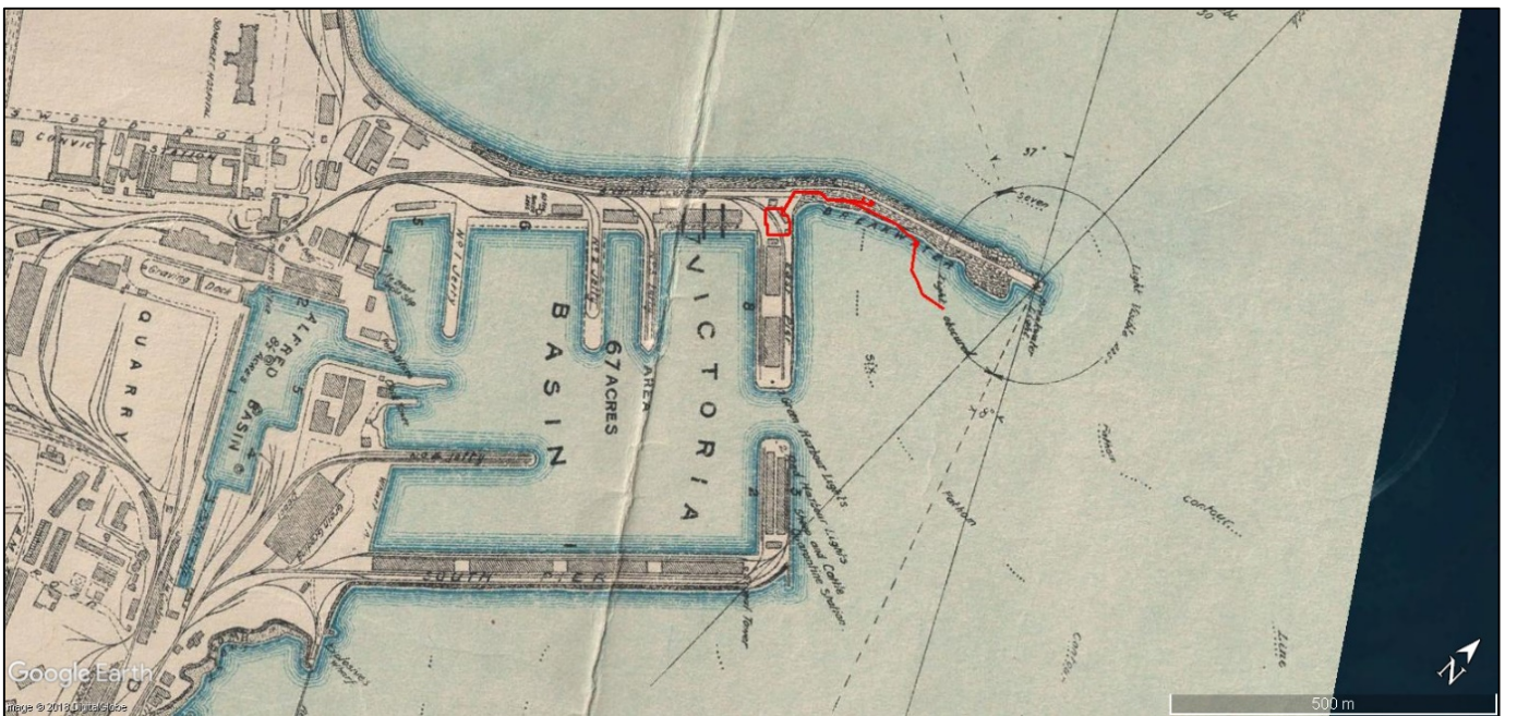
Figure 5.1.6: Proposed desalination plant infrastructure (red lines) superimposed onto portion of 1911 South African Railways map of Cape Town Harbour. Railway lines and buildings are now evident on the new harbour structures, and Victoria Basin has been named. Compared to 1900, harbour lights have been affixed at the ends of the breakwater and two piers, and the breakwater has been slightly extended inshore at its terminus. The terminus of the harbour rail line is indicated just to the north of the plant site, with two branch lines terminating at the end of East Pier, the easternmost of which traversing the plant site (Source: UCT Islandora 19899).
