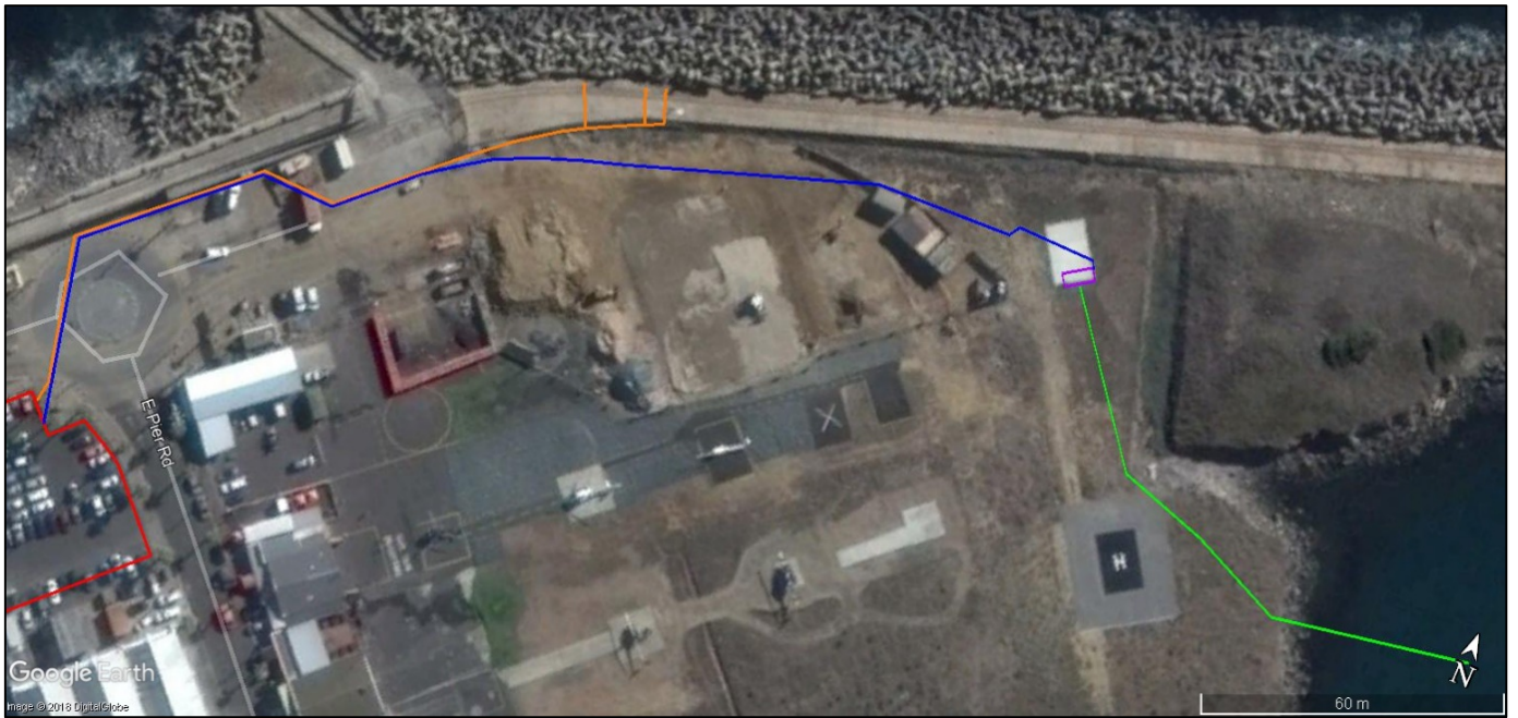
Figure 5.4.8: Proposed desalination plant site (red outline), marine abstraction structure (green line), pump house (purple rectangle) raw water intake pipeline (dark blue line) and brine outfall (orange line) indicated on 2017 satellite imagery (Google Earth 2017-05-19 dataset).
