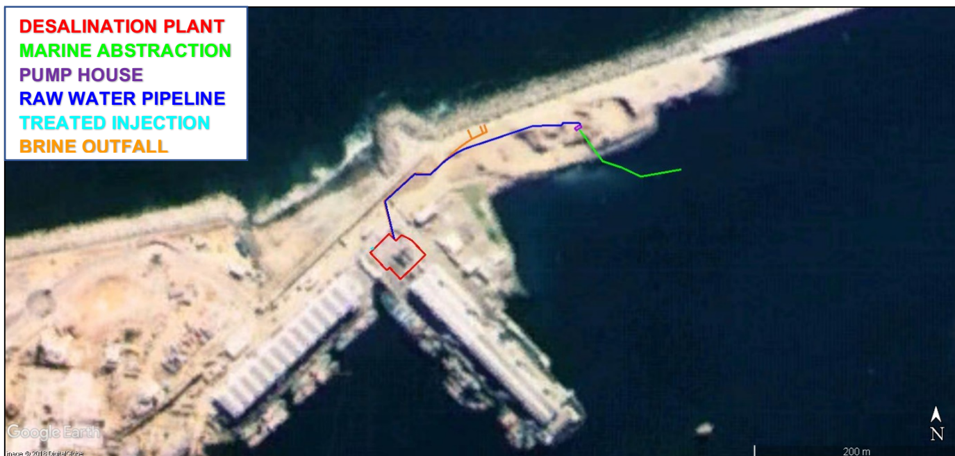
Figure 5.2.13: Proposed desalination plant infrastructure indicated on 1996 aerial photography. Dolosse now protect the breakwater and sea wall, and the reclamation of the area to the east and north-east of the plant site is progressing. Approximately half of the portion of marine abstraction pipeline currently proposed on land is already located on land (Source: Chief Directorate National Geo-spatial Information 994/96_3_31).
