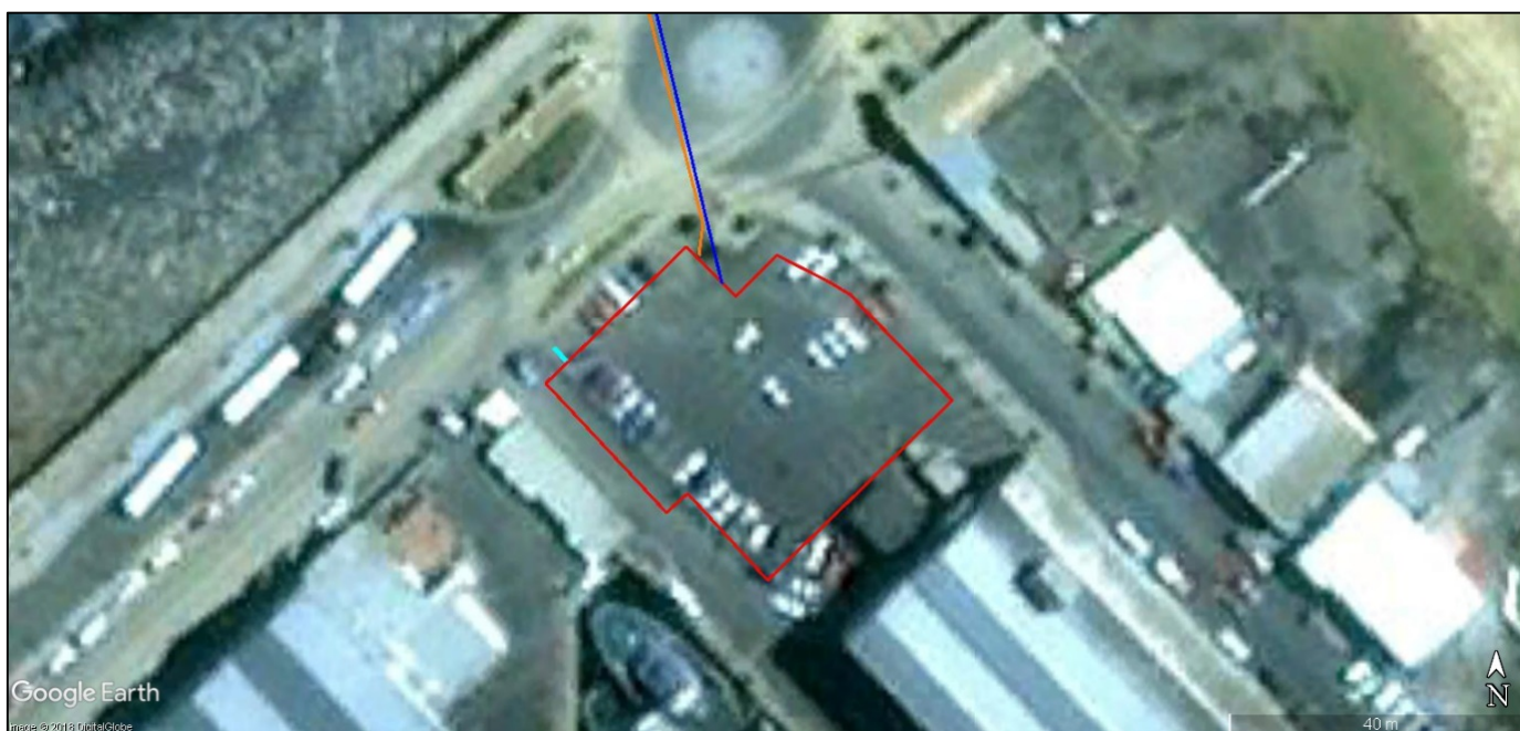
Figure 5.3.6: Proposed desalination plant site (red outline), raw water intake (dark blue line), treated water injection (dark blue line) and brine outfall (orange line) pipelines indicated on 2000 satellite imagery (Google Earth 2000-02-07 dataset).
