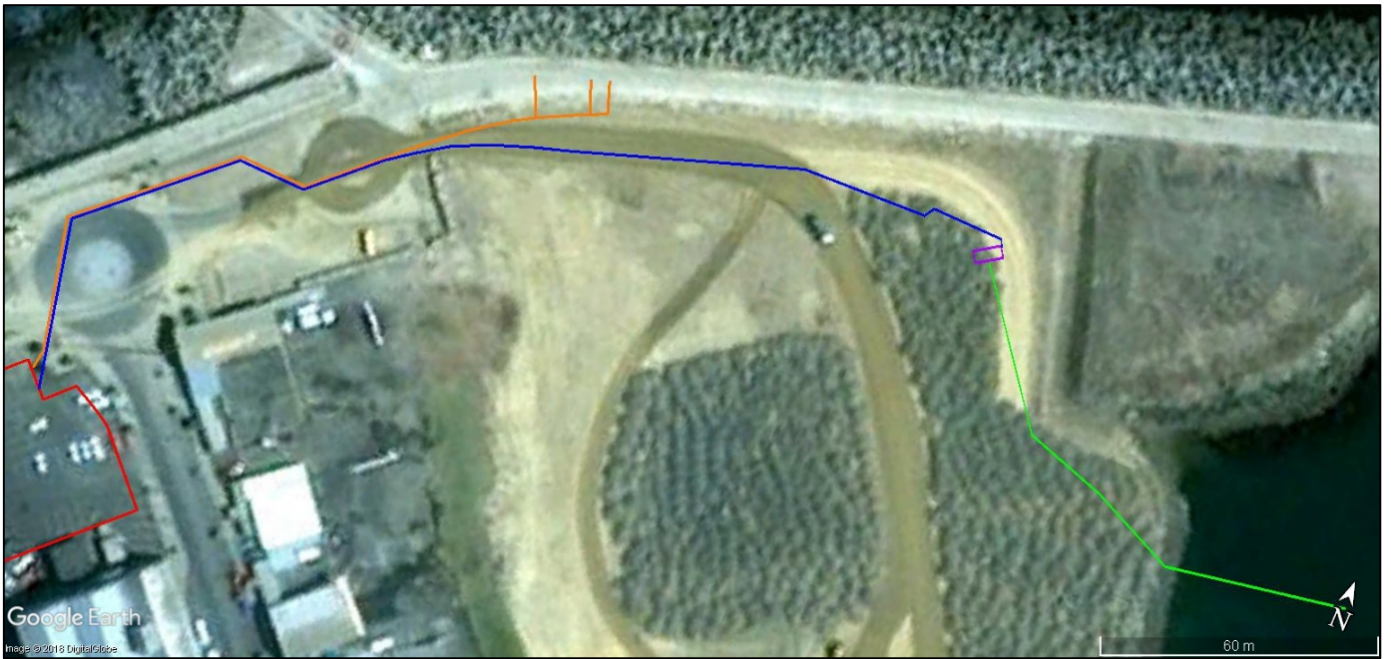
Figure 5.4.7: Proposed desalination plant site (red outline), marine abstraction structure (green line), pump house (purple rectangle) raw water intake pipeline (dark blue line) and brine outfall (orange line) indicated on 2000 satellite imagery (Google Earth 2000-02-07 dataset).
