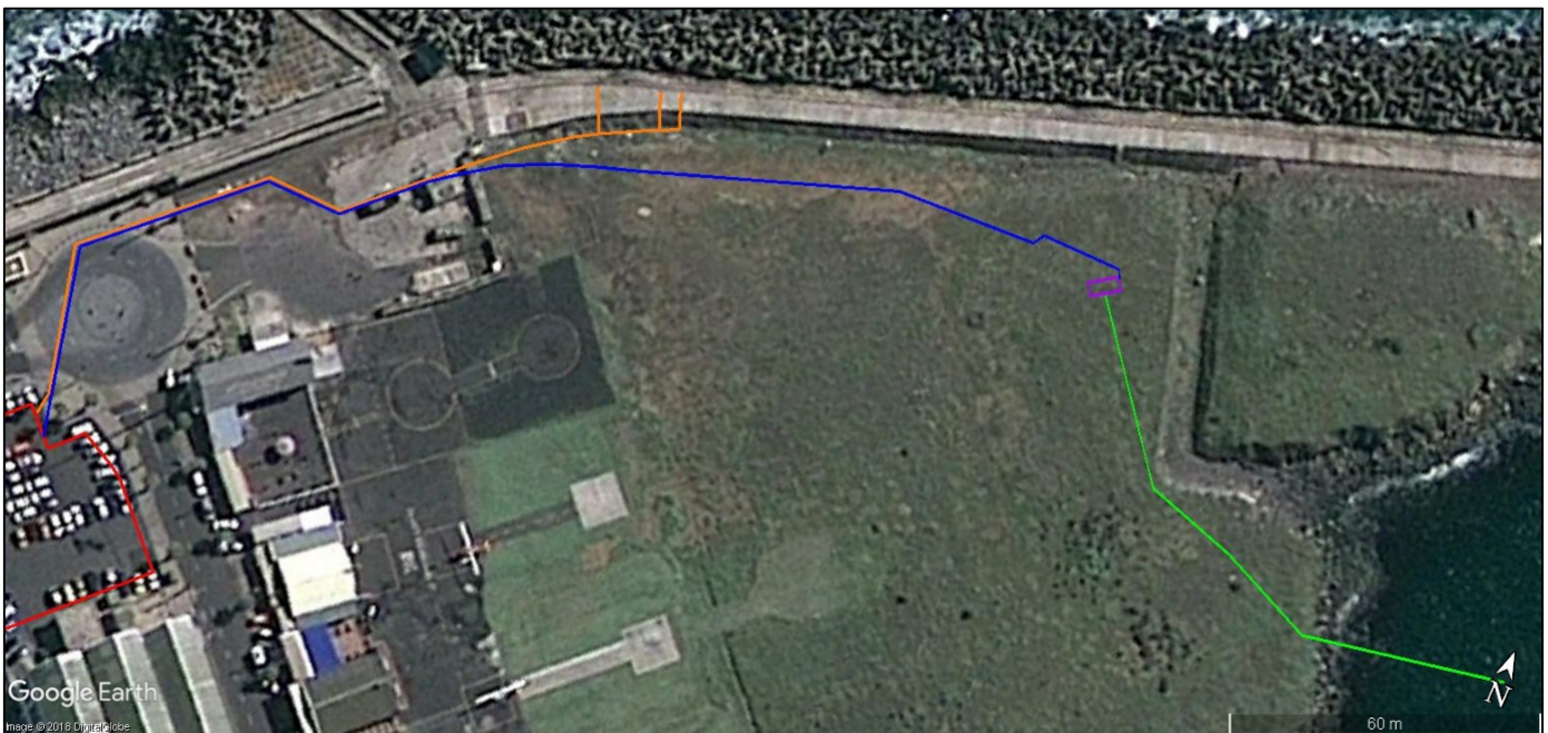
Figure 5.4.8: Proposed desalination plant site (red outline), marine abstraction structure (green line), pump house (purple rectangle) raw water intake pipeline (dark blue line) and brine outfall (orange line) indicated on (Google Earth 2009-09-11 dataset).
