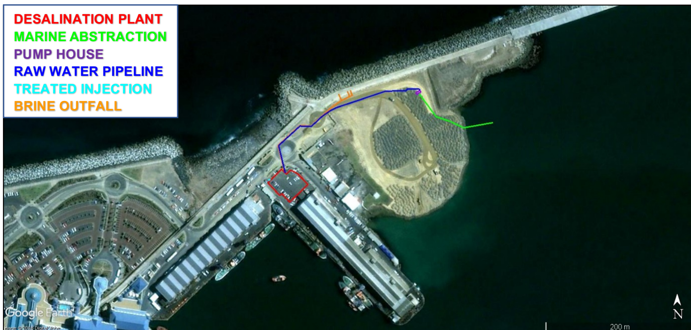
Figure 5.2.15: Proposed desalination plant infrastructure indicated on 2000 Google Earth satellite imagery. The proposed plant site has now become a parking area, and the rail lines have clearly made way for roads. The reclaimed area at the foot of the breakwater had reached its current extent, but the site is still in the process of establishment (Source: Google Earth 2000-02-07 imagery dataset).
