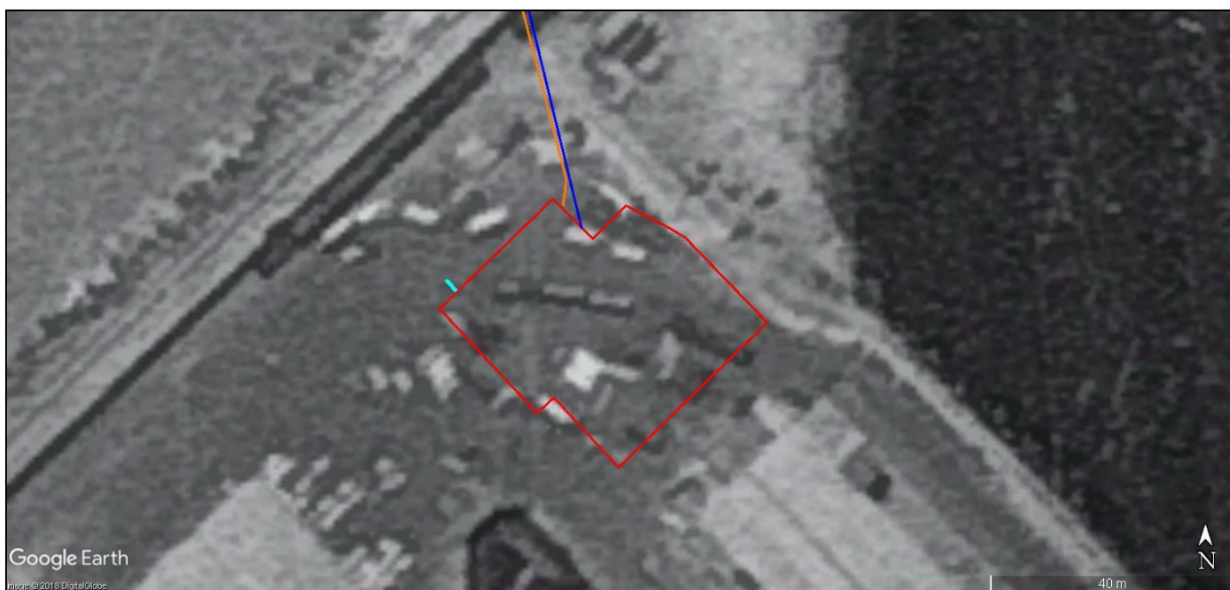
Figure 5.3.4: Proposed desalination plant site (red outline), raw water intake (dark blue line), treated water injection (dark blue line) and brine outfall (orange line) pipelines indicated on 1960 aerial photography (Source: Chief Directorate National Geo-spatial Information 454/60_18_7625).
