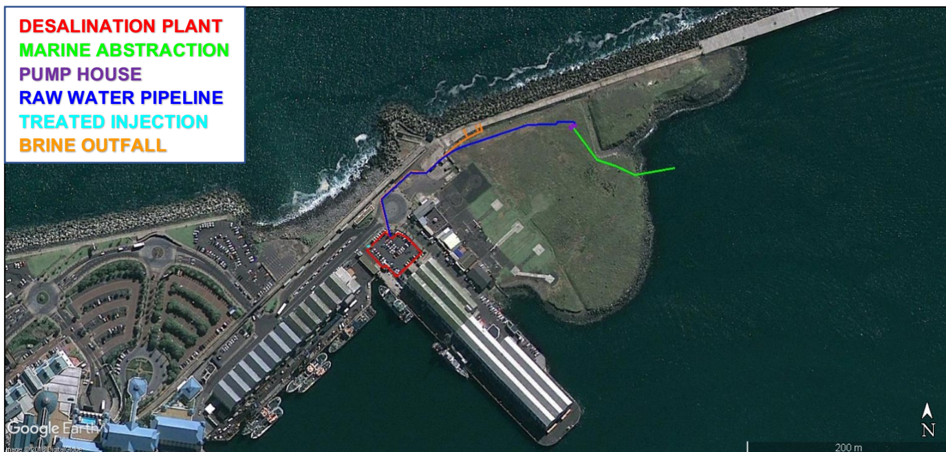
Figure 5.2.17: Proposed desalination plant infrastructure indicated on 2009 Google Earth satellite imagery. The reclaimed area has been stabilised and is largely vegetated. A number of new helicopter landing pads are visible on the western fringes of the reclaimed area. No buildings are located on the reclaimed area yet (Source: Google Earth 2009-09-11 imagery dataset).
