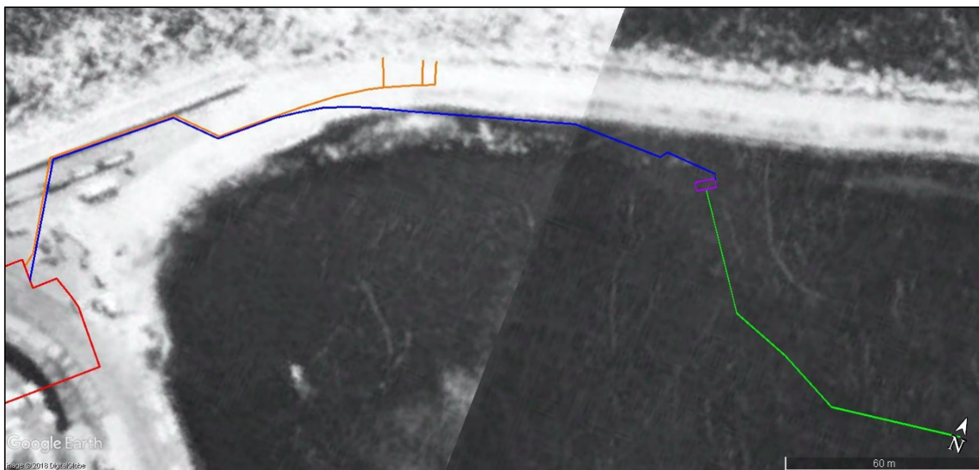
Figure 5.4.3: Proposed desalination plant site (red outline), marine abstraction structure (green line), pump house (purple rectangle) raw water intake pipeline (dark blue line) and brine outfall (orange line) indicated on 1945 aerial photography (Source: Chief Directorate National Geo-spatial Information 203A/45_4_618; _620).
