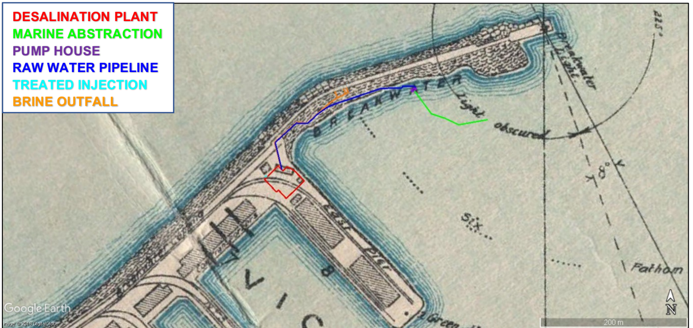
Figure 5.2.3: Proposed desalination plant infrastructure indicated on 1911 South African Railways map of Cape Town Harbour. Two large buildings on East Pier and number of smaller structures are now visible at the foot of East Pier, two of which are located within the proposed plant site. The site is traversed by a branch rail line to the end of East Pier. The seawall structure located to the north of the site is inscribed 'Breakwater capping', and the buildings to the south-west of the site 'Coal transporters' (Source: UCT Islandora 19899).
