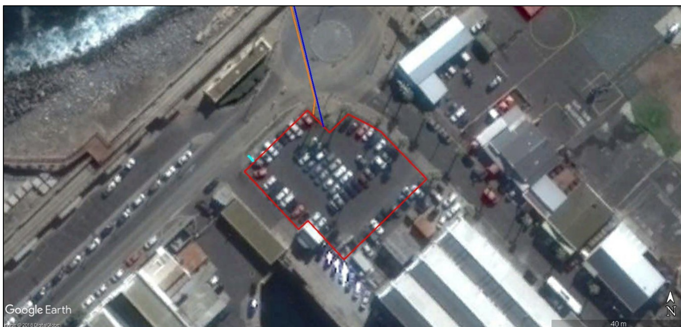
Figure 5.3.8: Proposed desalination plant site (red outline), raw water intake (dark blue line), treated water injection (dark blue line) and brine outfall (orange line) pipelines indicated on 2017 satellite imagery (Google Earth 2017-05-19 dataset).
