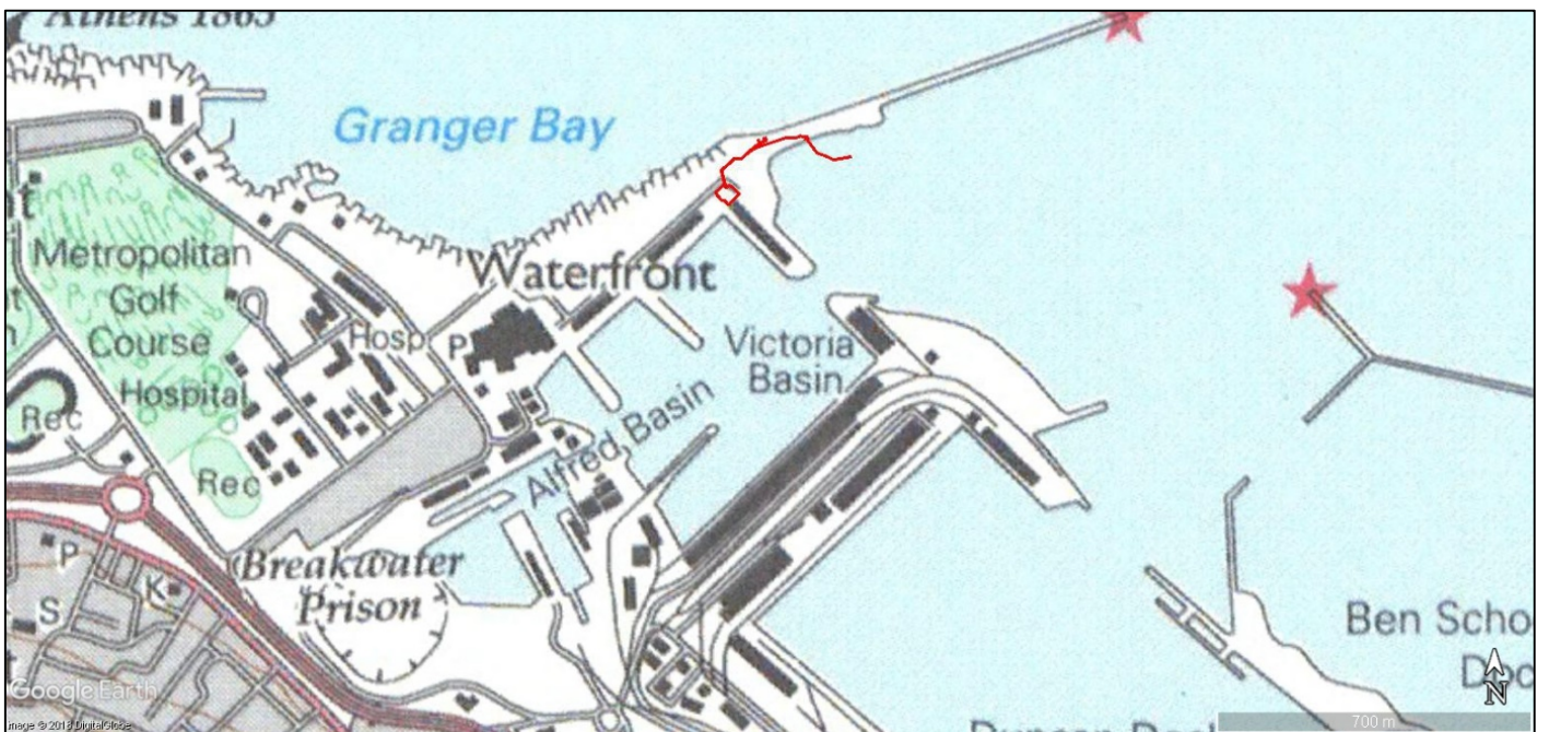
Figure 5.1.10: Proposed desalination plant infrastructure (red lines) superimposed onto portion of 1993 edition of Cape Town 3318CD 1: 50 000 topo-cadastral map. Compared to 1988, the (V&A) Waterfront has emerged, the railway lines have given way to roads, the oil sites have disappeared, and dolosse now protect the new seawall indicated on the 1988 map (Source: Chief Directorate National Geo-spatial Information).
