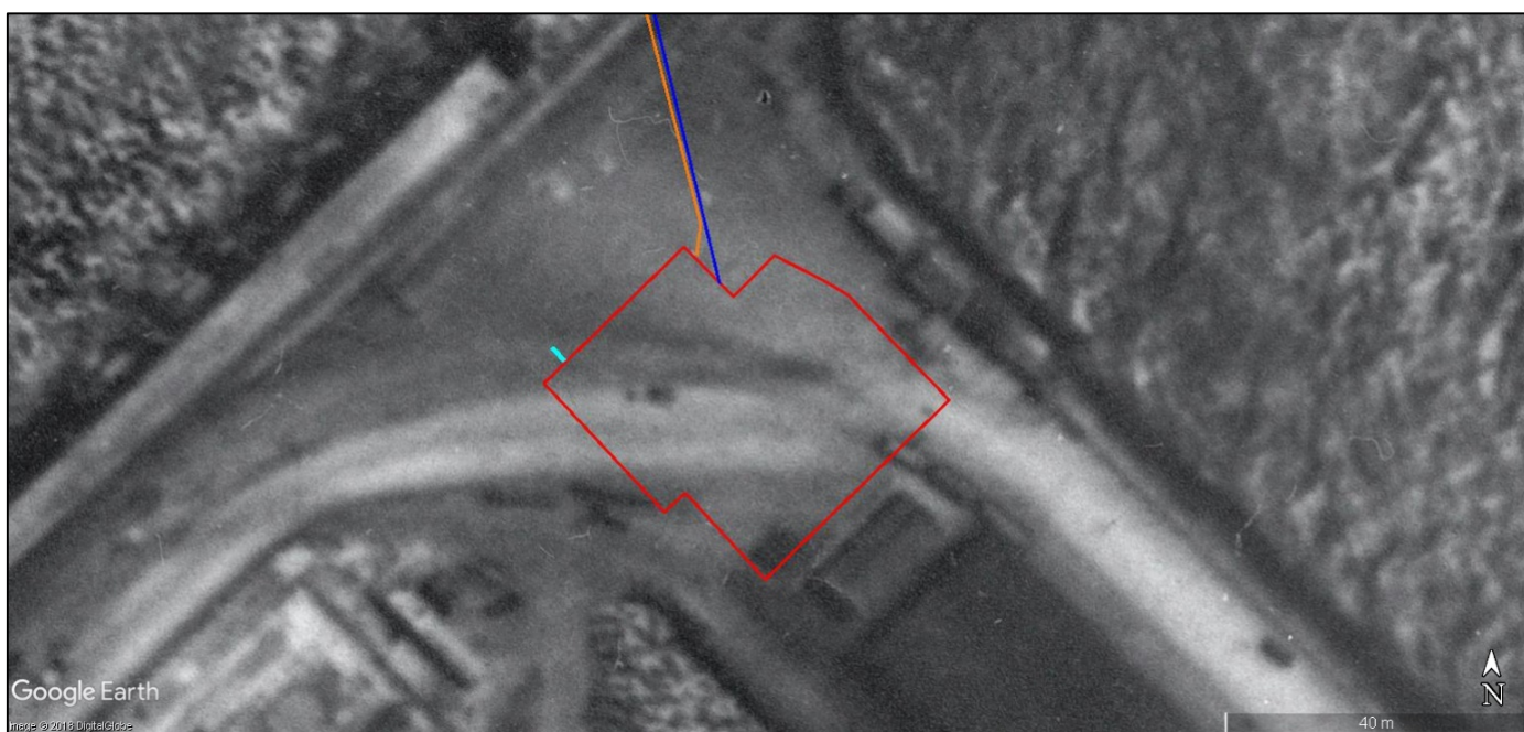
Figure 5.3.2: Proposed desalination plant site (red outline), raw water intake (dark blue line), treated water injection (dark blue line) and brine outfall (orange line) pipelines indicated on 1926 aerial photography (Source: Chief Directorate National Geo-spatial Information 1926_05_0855; _0859).
