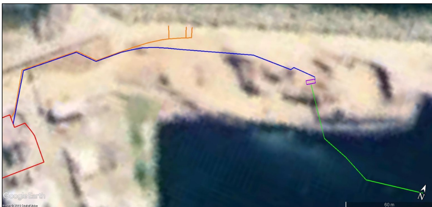
Figure 5.4.6: Proposed desalination plant site (red outline), marine abstraction structure (green line), pump house (purple rectangle) raw water intake pipeline (dark blue line) and brine outfall (orange line) indicated on 1996 aerial photography (Source: Chief Directorate National Geo-spatial Information 994/96_3_31).
