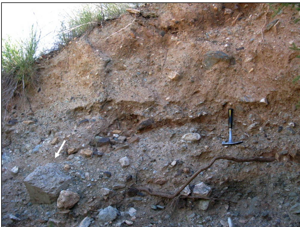
Fig. 5. Poorly-sorted, well-bedded alluvial sediments adjacent to footings of Bridge 3 (Hammer = 32 cm). Inclusions of concrete (arrow) show that this is in fact an artificial deposit.
