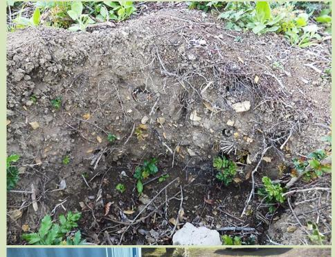
Left: A pit 500mm square excavated in the middle of the site showing the composition of the topsoil overburden – note the brown siltstone flakes. This hole was possibly dug to remove a root stock of a bush that was removed.
