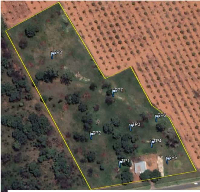
Figure 29: Positions of geotechnical test pits marked TP1 - TP8
