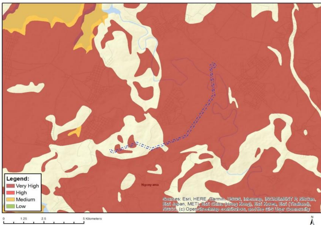
Figure 30: Provisional palaeosensitivity mapping of the Grid Connection project area using the DFFE Screening Tool (image provided by CES). The Very High palaeosensitivity of much of the project area (dark red) is contested here. Insensitive areas are underlain by Karoo dolerite.
