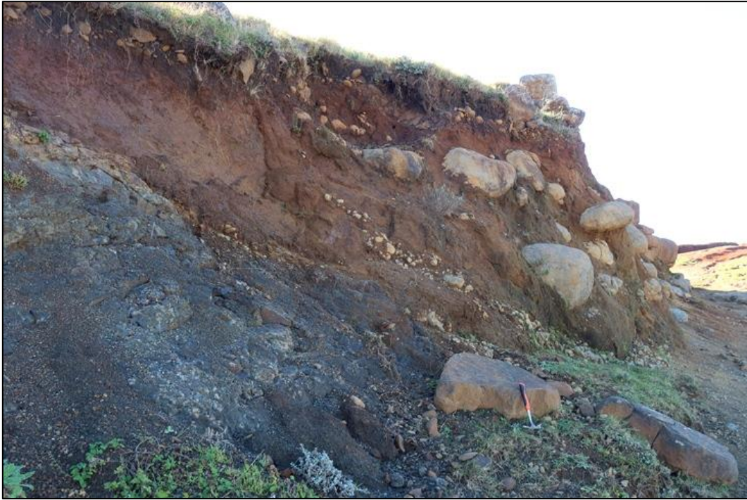
Figure 21: Escarpment edge quarry area on Farm RE/101 exposing weathered, dark grey Burgersdorp Formation mudrocks overlain by a possible colluvial channel infill with suspended, rounded dolerite corestones (hammer = 30 cm).
