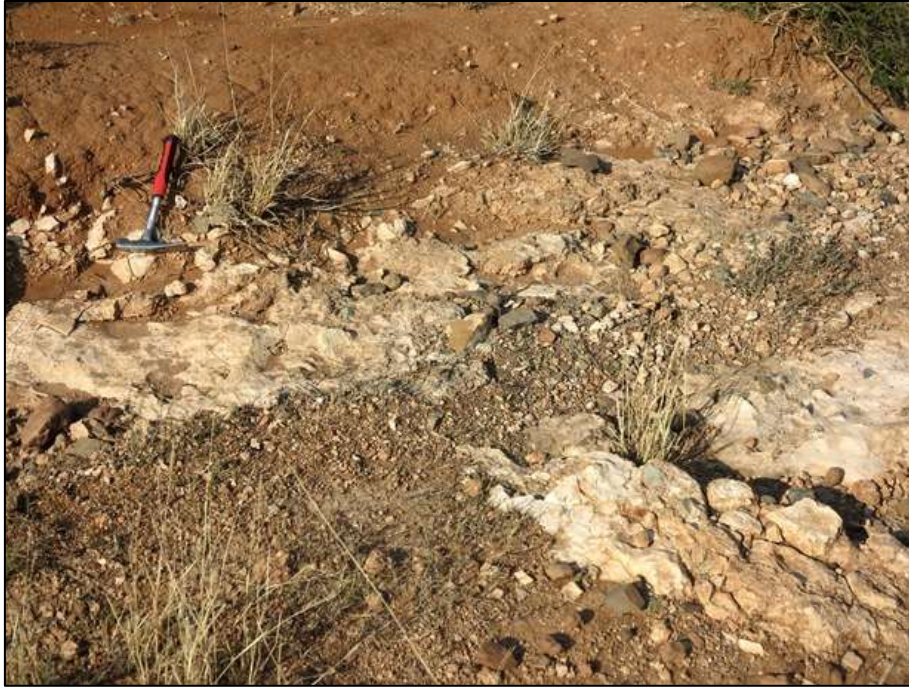
Figure 30: Thin, locally gravel-rich calcrete hardpan beneath semi-consolidated, orange-brown sandy alluvium exposed in a shallow stream bank, eastern sector of the Tango WEF project area (hammer = 30 cm).
