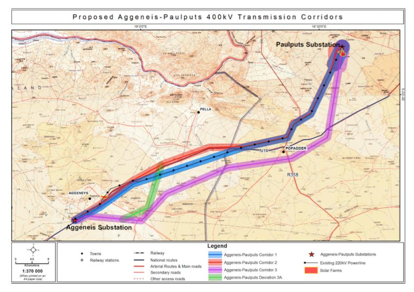
Figure 1: Map showing the three route options (Corridors 1, 2 & 3 with possible deviation 3A) under consideration for the proposed new 400 kV transmission line between the existing Aggeneis and Paulputs Substations, Namaqua and Siyanda Districts, Northern Cape. Corridor 1 is the preferred route option and largely follows an existing 220 kV powerline and associated access road (black line with dots).
