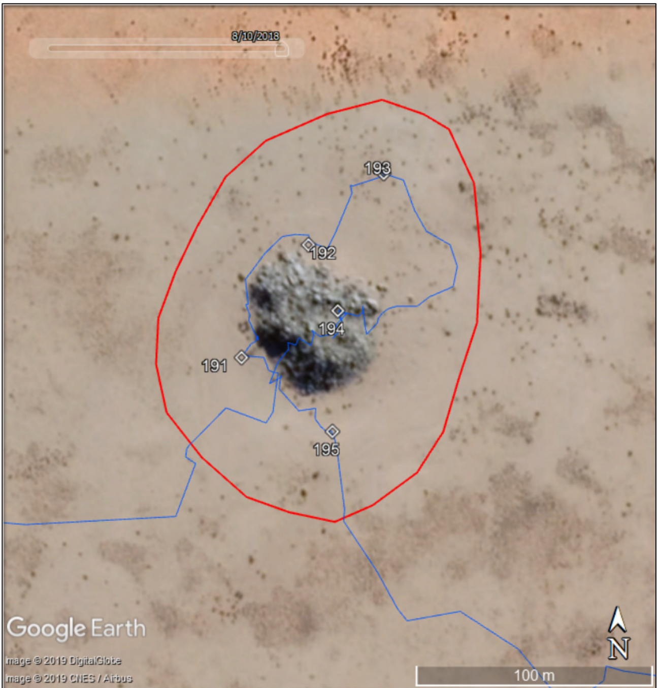
Figure A3.2: Map of the area around the rocky hill showing the survey tracks (blue lines), the recorded finds (numbered white symbols) and a no-go buffer of 30 m (red outline).
