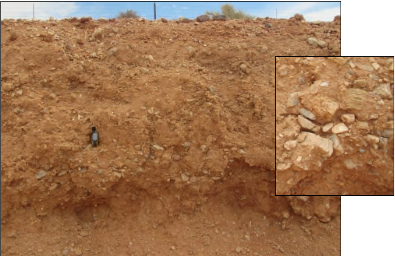
Figure 8: View of the section in the borrow pit that lies alongside the Loop 10 gravel road near the site. The inset shows the sub-angular clasts that dominate the profile.
