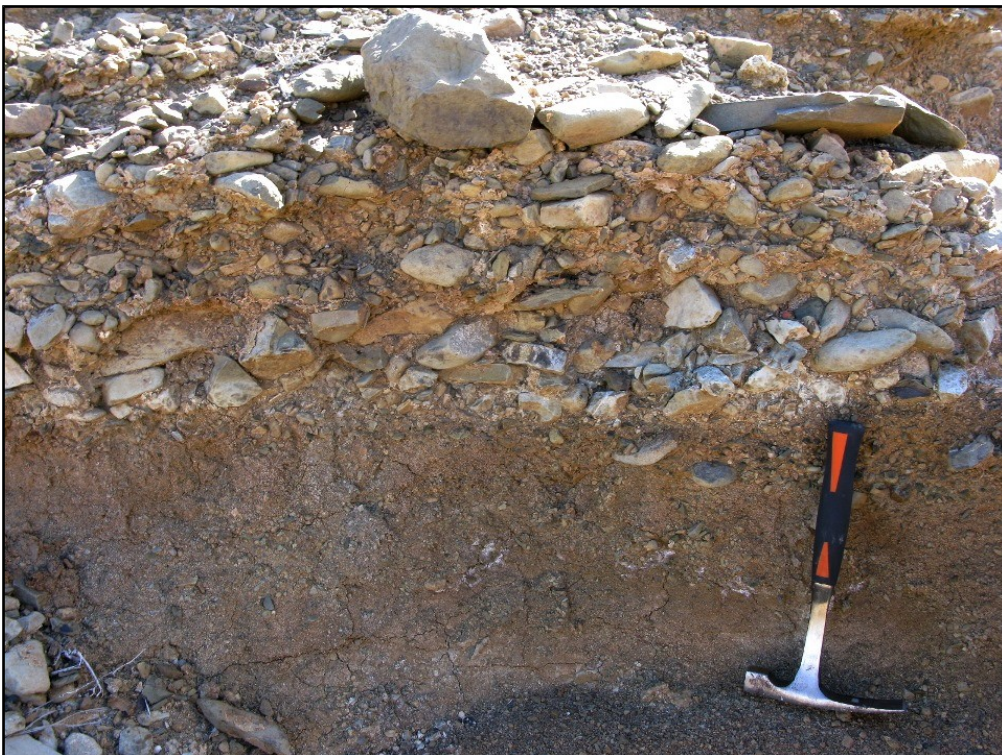
Fig. 7. Silty to sandy alluvium sharply overlain by a horizon of coarse, clast-supported gravels, locally showing current imbrication, pit site MR00374/2.4/0.1R (Hammer = 30 cm).
