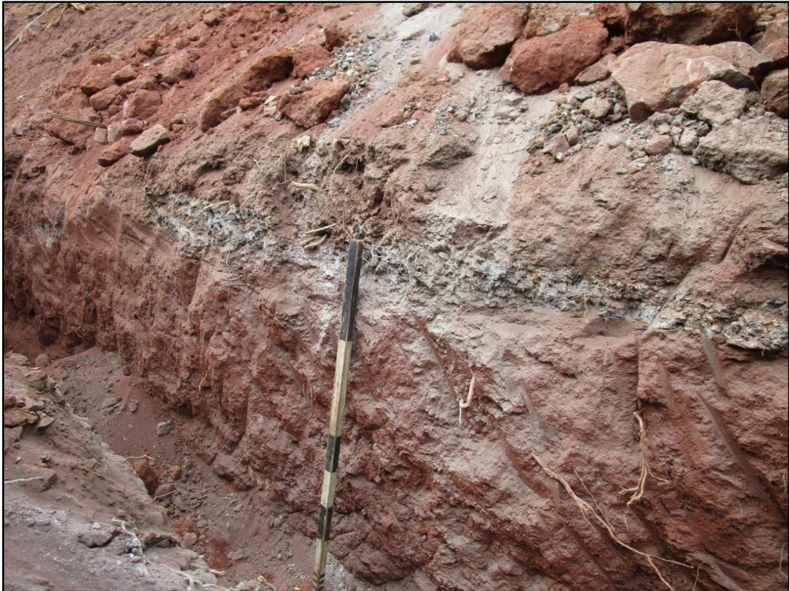
Figure 7. View of the profile of the trench indicating a coal fire ash layer at the top.
