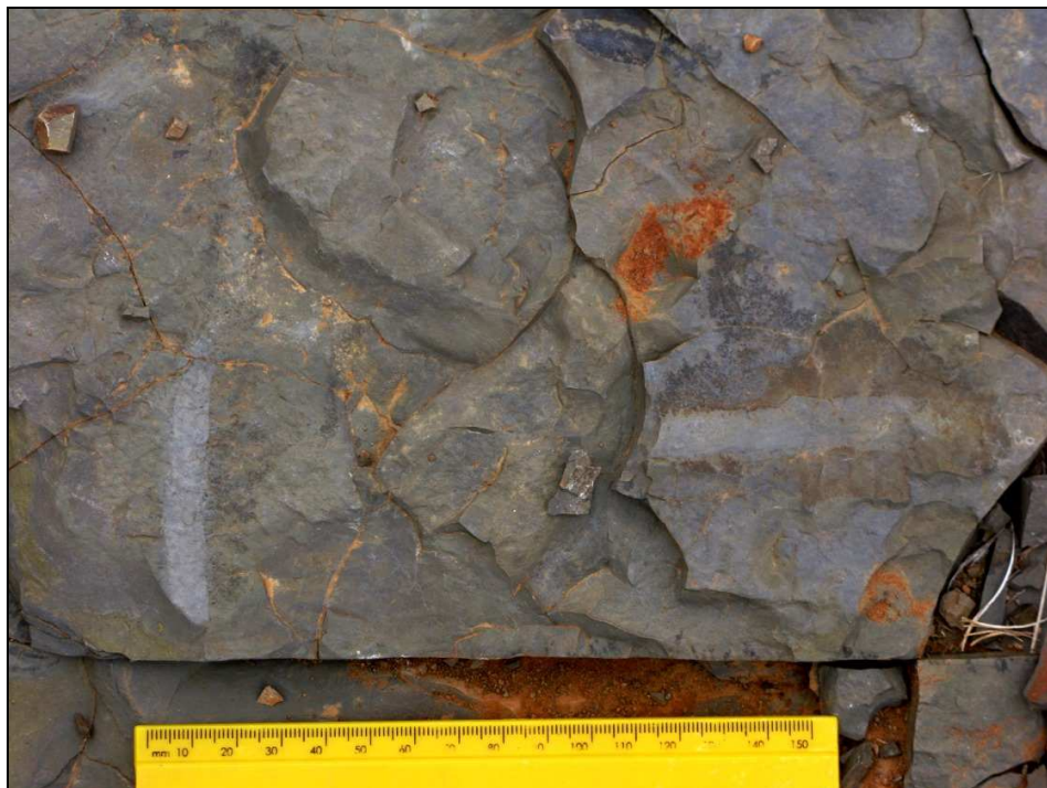
Fig. 14. Dark grey, baked Tierberg-like Ecca mudrocks containing abundant flattened horizontal burrows up to 1 cm across, Loc. 271 (Scale in cm and mm).
