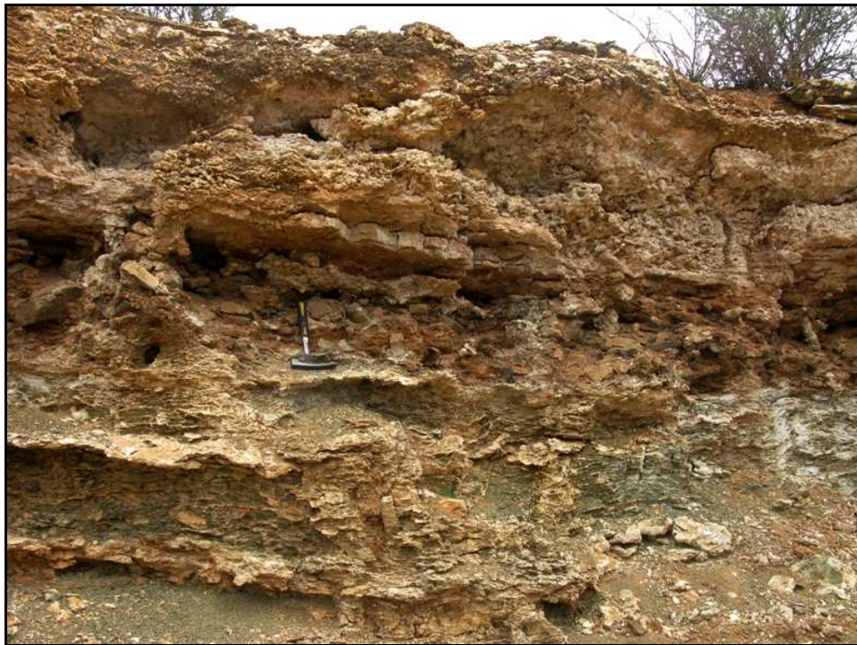
Fig. 23. Composite, multi-layered calcrete hardpan with coarse gravel horizon adjacent to hammer, quarry exposure near N10 (Q4 in Fig. 2) (Hammer = 30 cm).
