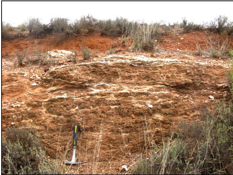
Fig. 22. Well-consolidated, calcretised older alluvial soils overlain by unconsolidated orange-brown younger soils, quarry exposure in southern part of the study area (Q1 in Fig. 2) (Hammer = 30 cm).
