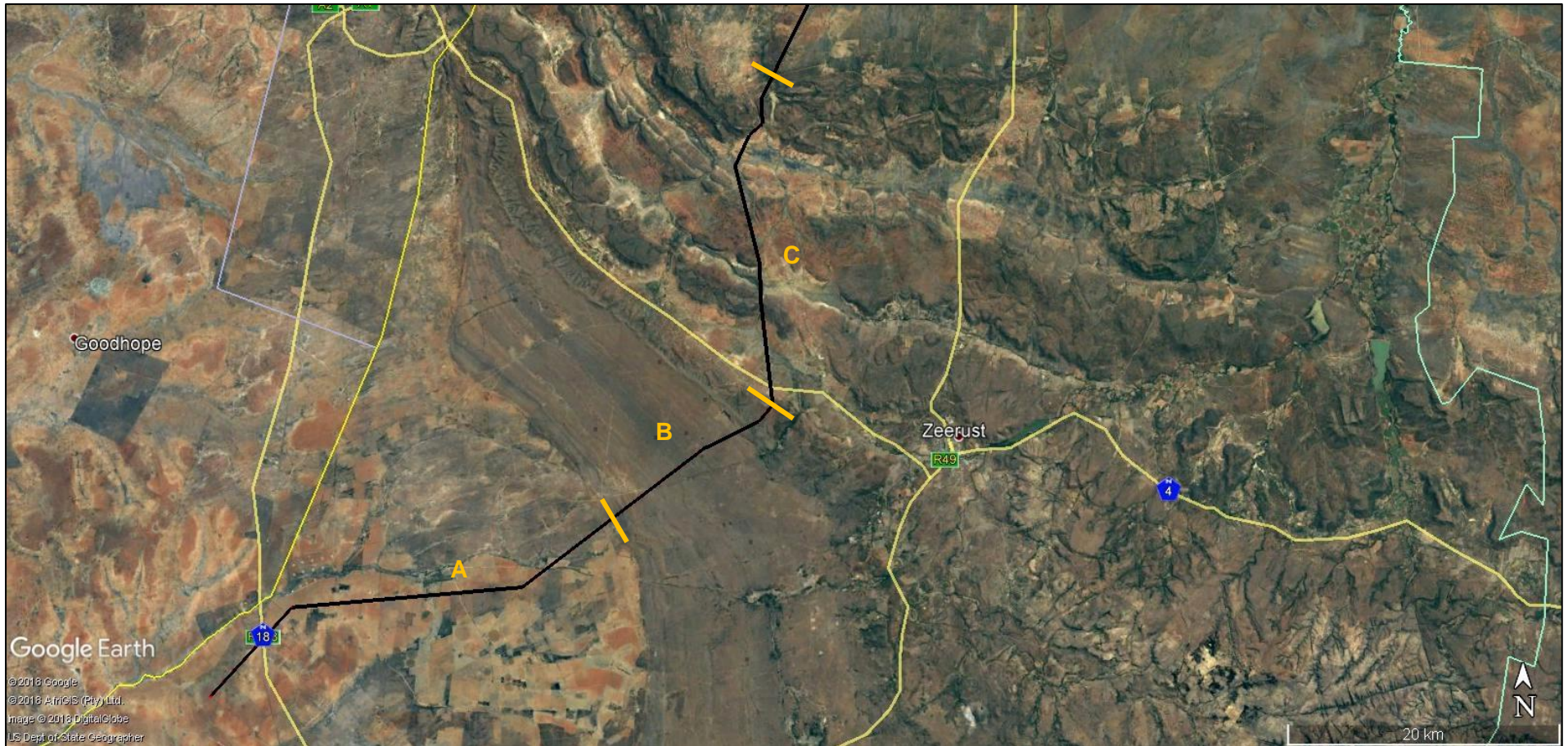
Figure 2. Google earth© satellite image of BOSA 400 kV transmission line geological Sectors A, B and C, North West Province, South Africa. Dark yellow line = RSA / Botswana Border. Black line = BOSA transmission line corridor.
