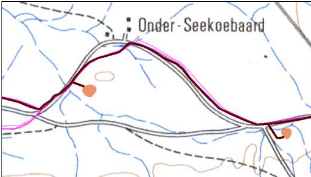
Figure A3.2: Map showing the two existing borrow pits in orange along the southern side of the access road to the hydro-electric site. Their maximum dimensions are currently 90 m and 70 m respectively.
