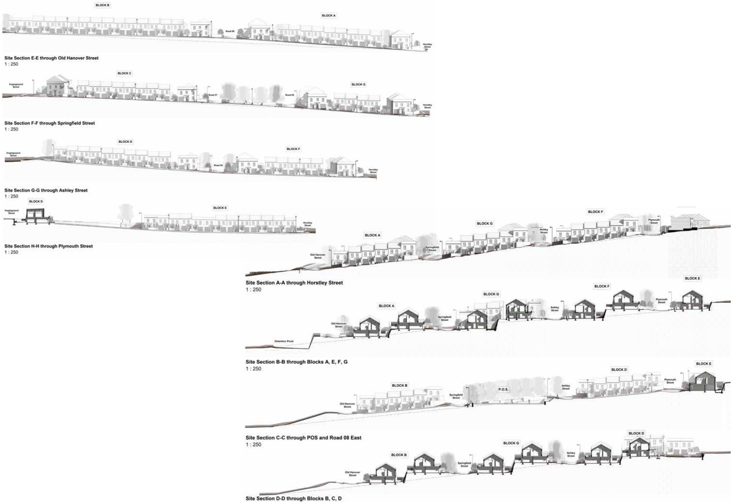
Figure 15. Sections through site showing the extent of cut and fill necessary to create the patforms for construction (D6 ADE-JV, 2022)
