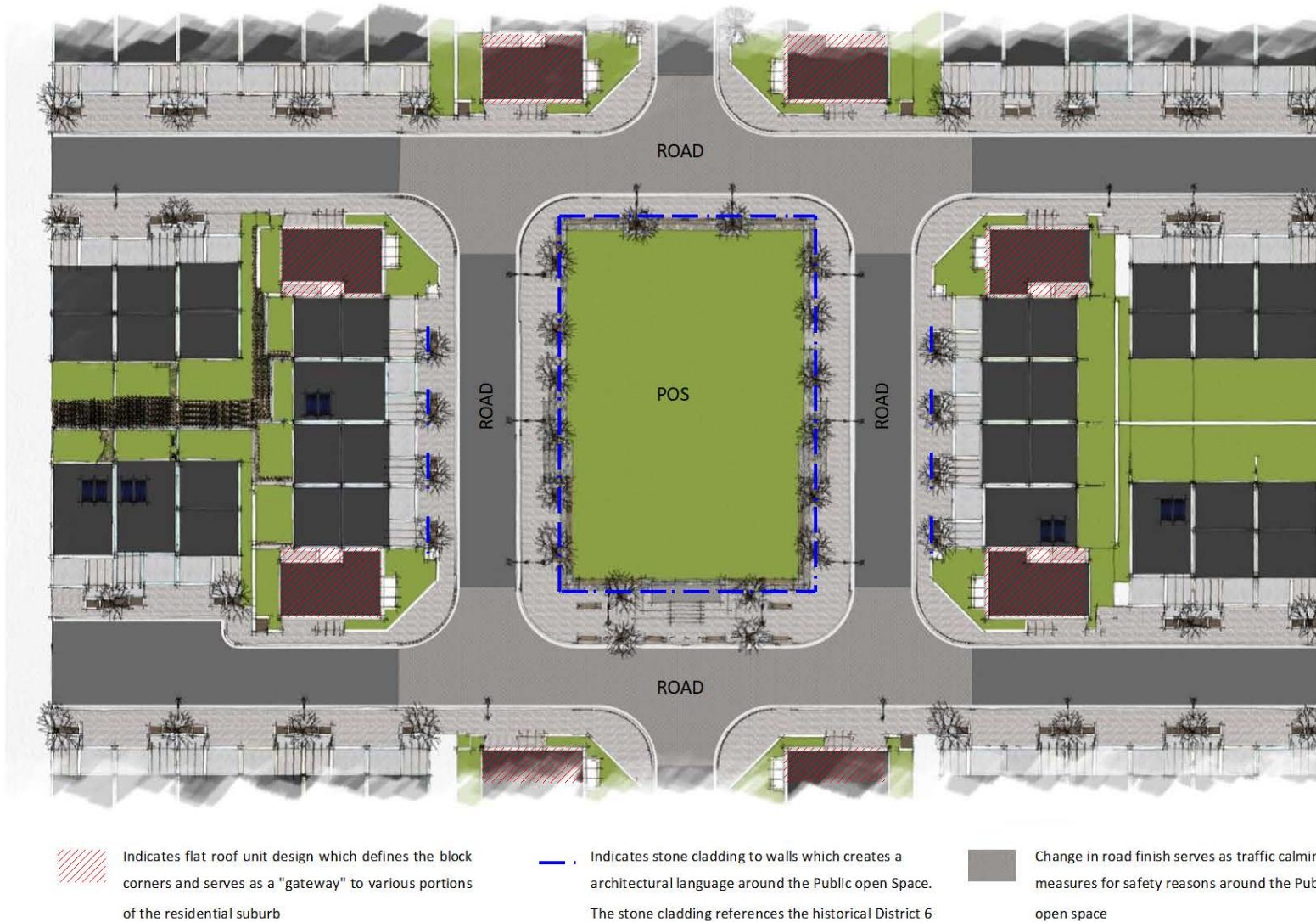
Figure 2.6.4: Plan of proposed layout arranged around a central public open space
