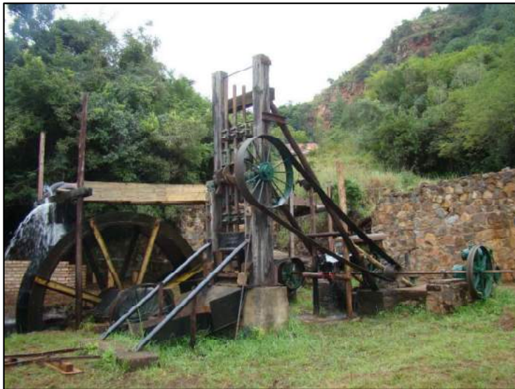
Figure 6-23: An archive photo of the water wheel and stamping battery dating to 2005 (Pistorius).
