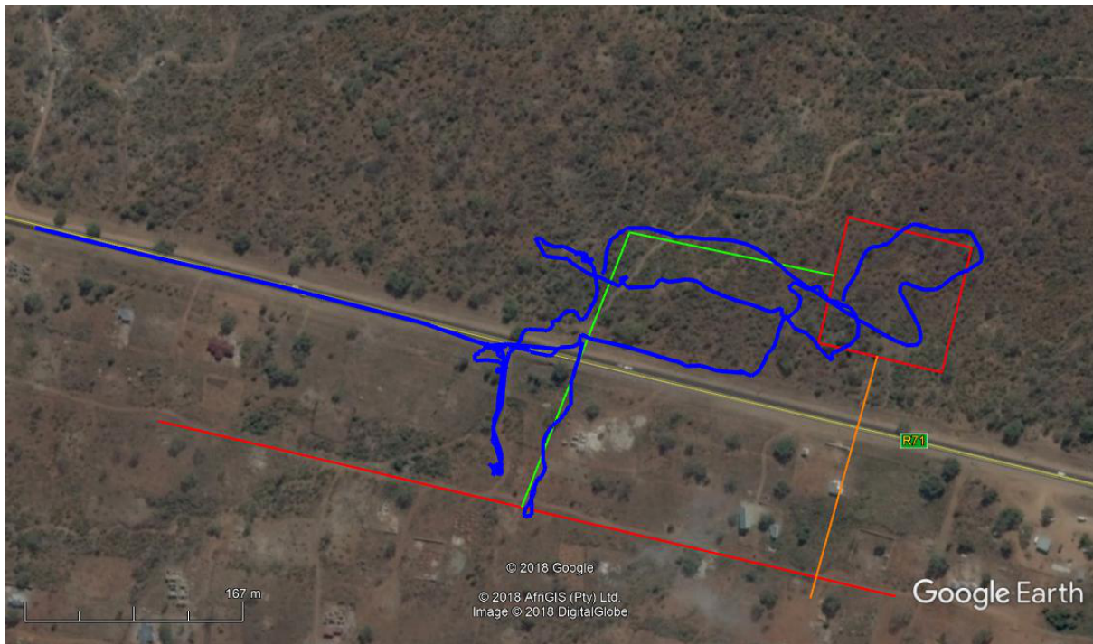
Figure 4: GPS track of the field survey (blue lines). North reference is to the top. The green line represents the proposed new power line, the orange the authorised one and the red square the area for the authorised substation.
