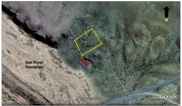
Figure 10. Google satellite indicating location of Sites 1 and 2 and the boundary of the proposed borrow pit (yellow polygon). The red polygon is the proposed laydown area. The yellow line is the proposed 250m long access road
