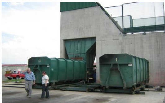
(c) Front view with roll-on bins into which waste is compacted.
