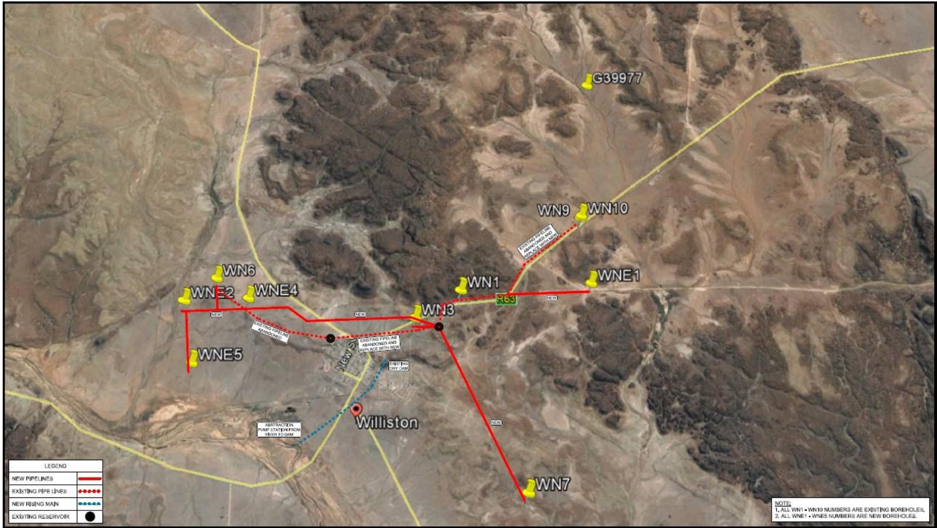
Figure 1. Outline of the proposed potable water supply infrastructure near the town of Williston, Northern Cape (Image prepared by Lyners Consulting Engineers, George). Solid red lines indicate new pipelines, the blue dotted line is the new rising main, while new and existing boreholes are marked by yellow tick symbols.
