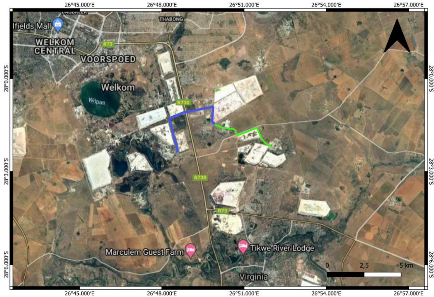
Figure 1: Google Earth (2021) Image indicating the locality of the proposed new reclamation pump station at FSS 6 TSF and slurry transfer line from FSS6 TSF to Saaiplaas Plant. New transfer line is indicated in blue and existing line in green
