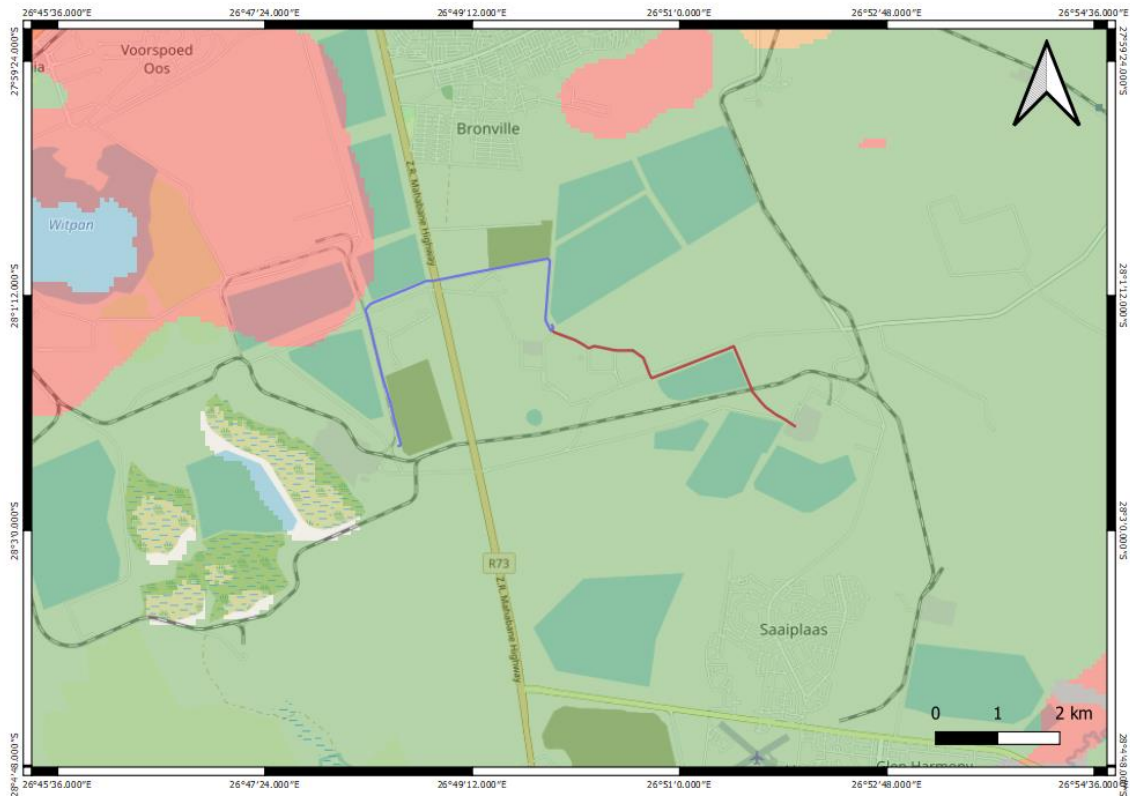
Figure 5 - Extract of the 1 in 250 000 SAHRIS PalaeoMap map (Council of Geosciences) indicating the proposed development in blue and the existing pipeline in red.
