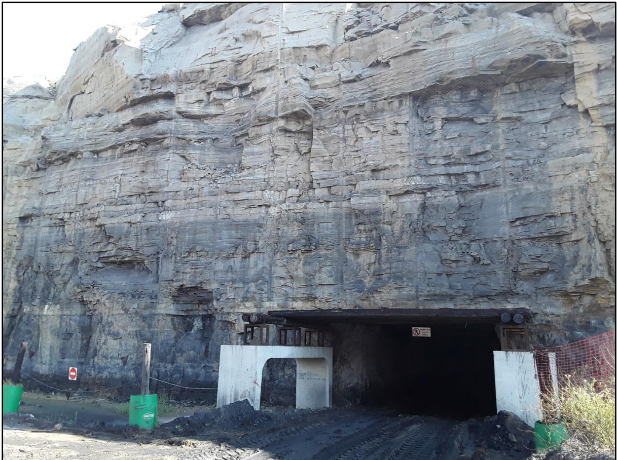
Figure 3: Adit to the underground mine on the farm Groenkloof 40 IT (TZP4), in Mpumalanga, South Africa.
