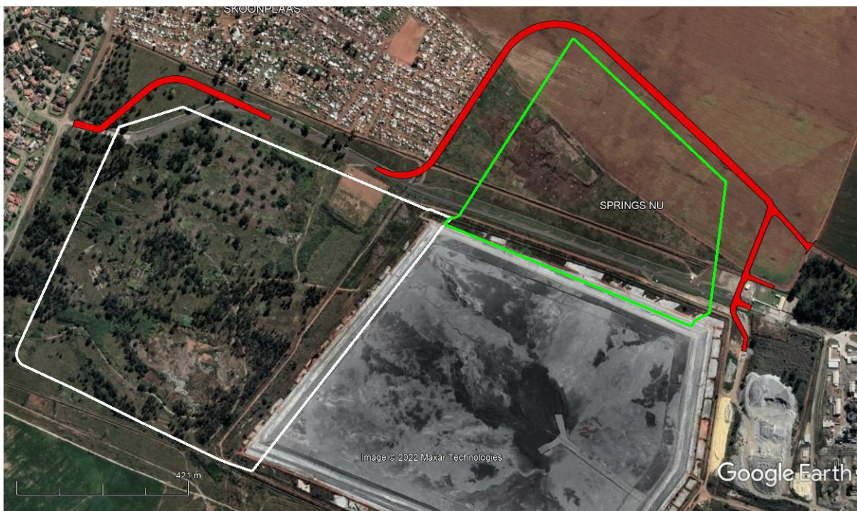
FIGURE 3: PROPOSED SITES FOR THE DEVELOPMENT. THE TSF EXPANSION WEST IS IN THE WHITE BORDER AND THE TSF EXPANSION NORTH IN THE GREEN BORDER.
