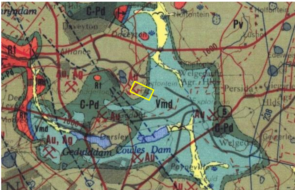
Figure 3: Geological map of the area around the Modder East Operations mine within the yellow rectangle. Abbreviations of the rock types are explained in Table 2. Map enlarged from the Geological Survey 1: 250 000 map 2628 East Rand.
