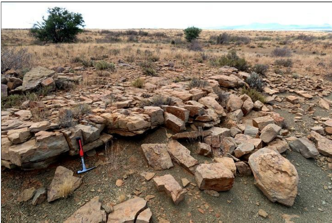
Figure 45: Thin, well-jointed channel sandstone of the Lower Beaufort Group (hammer = 30 cm).
