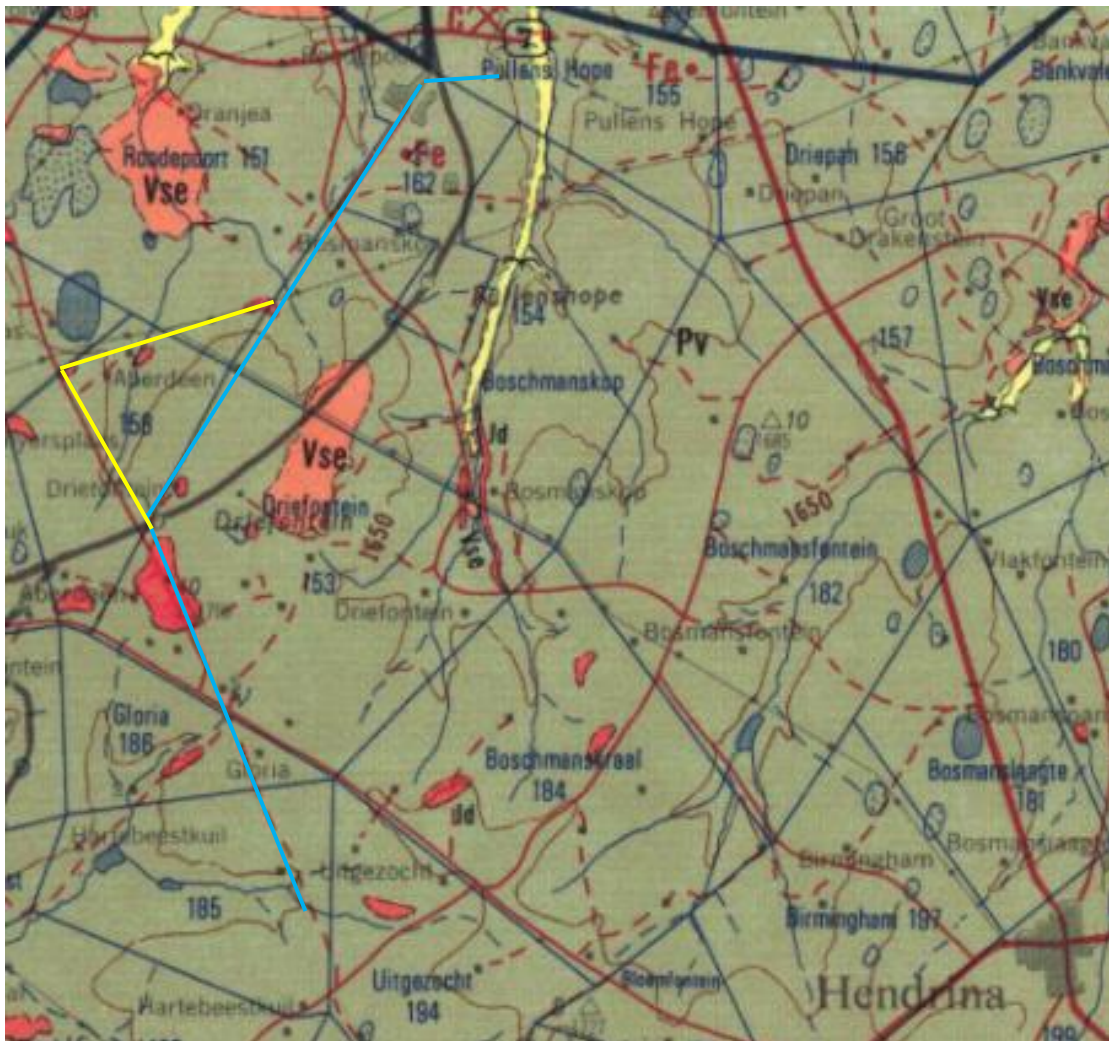
Figure 2: Geological map of the area around the Hendrina Substation and proposed power lines. Blue line is the preferred route and yellow line the alternate route. The location of the proposed project is indicated within the yellow rectangle. Abbreviations of the rock types are explained in Table 2. Map enlarged from the Geological Survey 1: 250 000 map 2628 East Rand.
