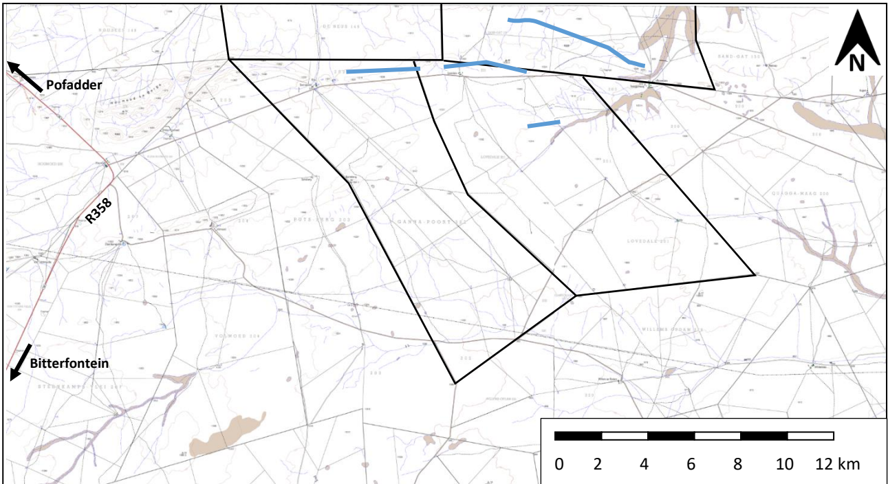
Figure 1: Extract from 1:50 000 topographic mapsheets 2918BC and 2918BD showing the location of the site. Black polygons show farm portions, blue lines show the turbine rows. Source of basemap: Chief Directorate: National Geo-Spatial Information. Website: www.ngi.gov.za .
