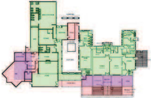
Fig. K: Positive and negative elements clubhouse building – position of possible demolitions, additions/alterations.
