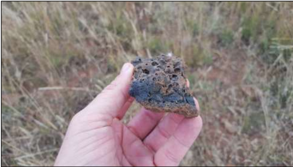
Figure 5-8: Metal smelting residue (slag) from Site EXIGO-DFM-IA02.
