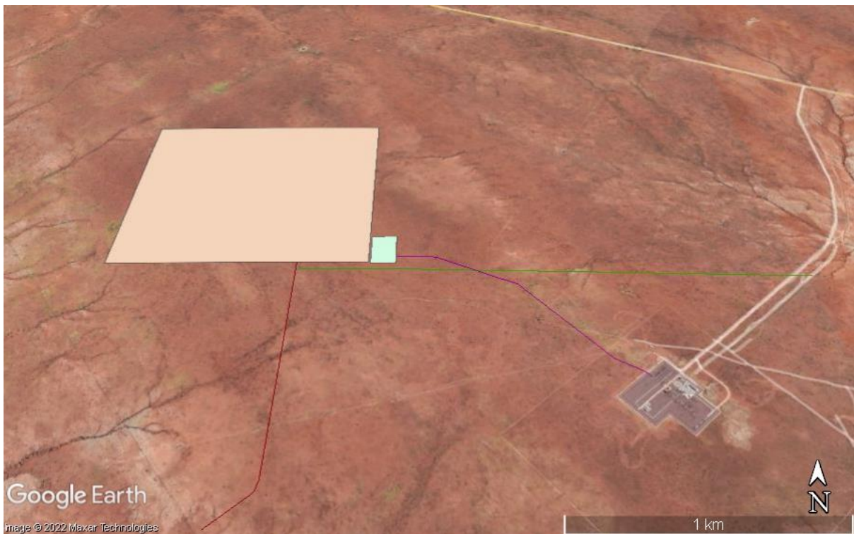
Figure 2: Google Earth Map of the proposed Site A option for the Kiwano BESS and PV facility, south of the road to Lutzputs and close to the Kiwano Substation. Pale pink polygon = site boundary site; green polygon = substation; red line = access road; green line = pipeline; purple line = powerline.
