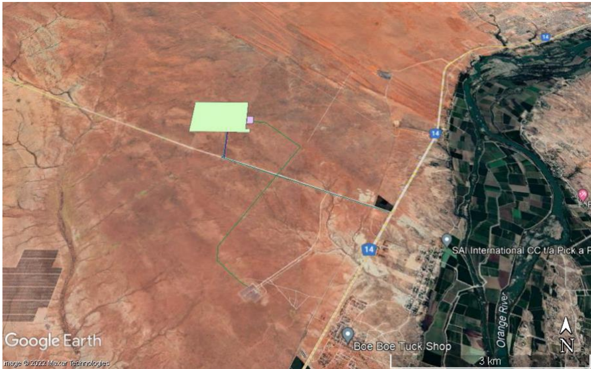
Figure 3: Google Earth map of Site B alternative for the Kiwano BESS and PV facility; Green polygon = site boundary; lilac polygon = substation; green line = powerline; blue line = pipeline and purple line = access road. Note this option is north of the road to Lutzputs and farther away from the existing Kiwano Substation.
