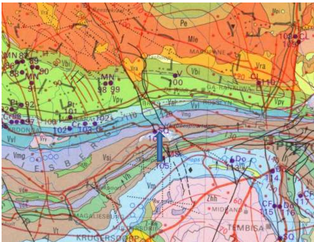
Figure 2: Geological map of the area around the Hartebeespoort Dam. The location of the proposed project is indicated with the arrow. Abbreviations of the rock types are explained in Table 2. Map enlarged from the Geological Survey 1: 1 000 000 map 1984.
