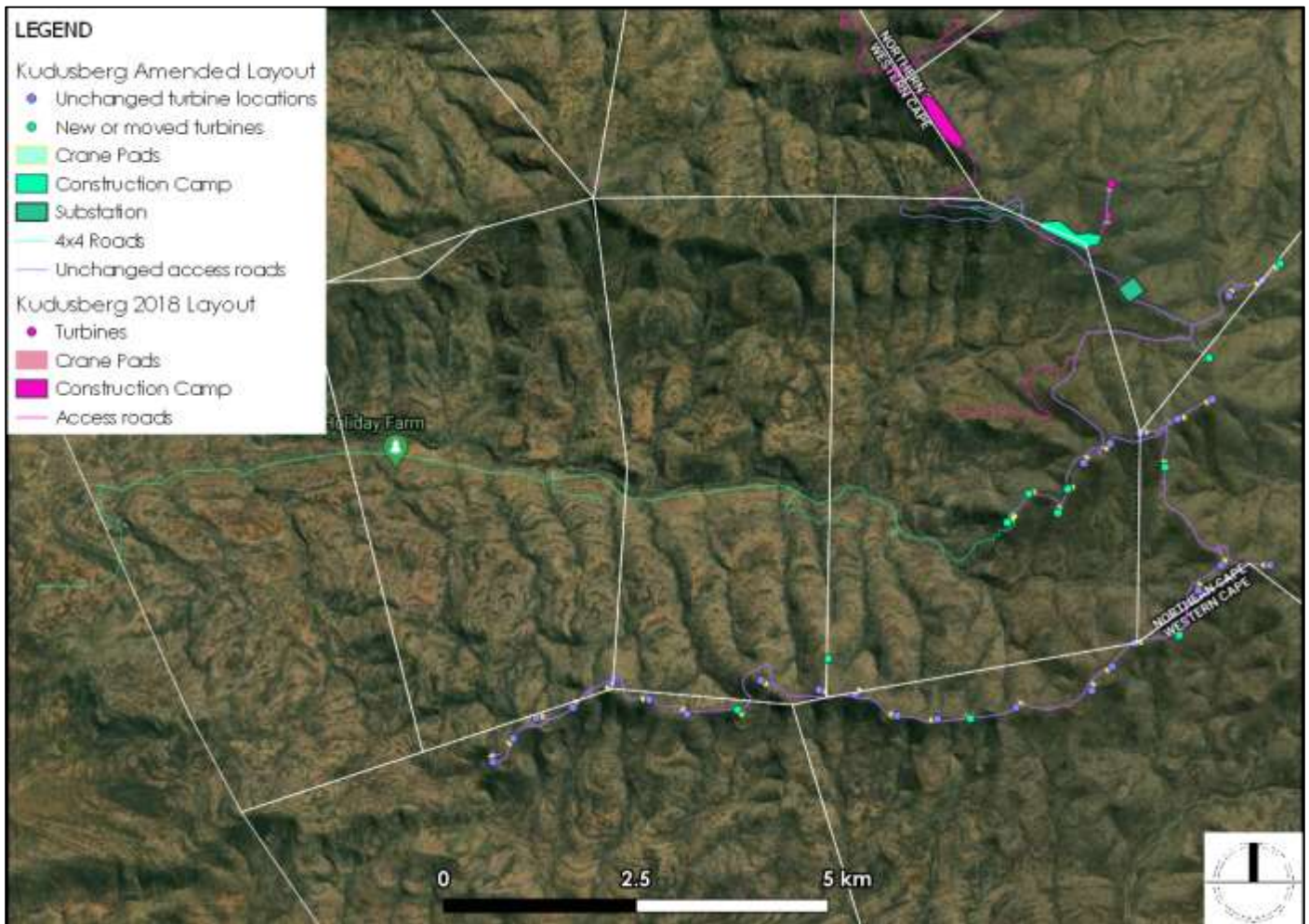
Figure 2. The newly proposed Kudusberg WEF layout overlaid on the original layout showing the minor differences proposed; all visible Kudusberg 2018 turbines will be relocated or removed (RSA, 2021).
