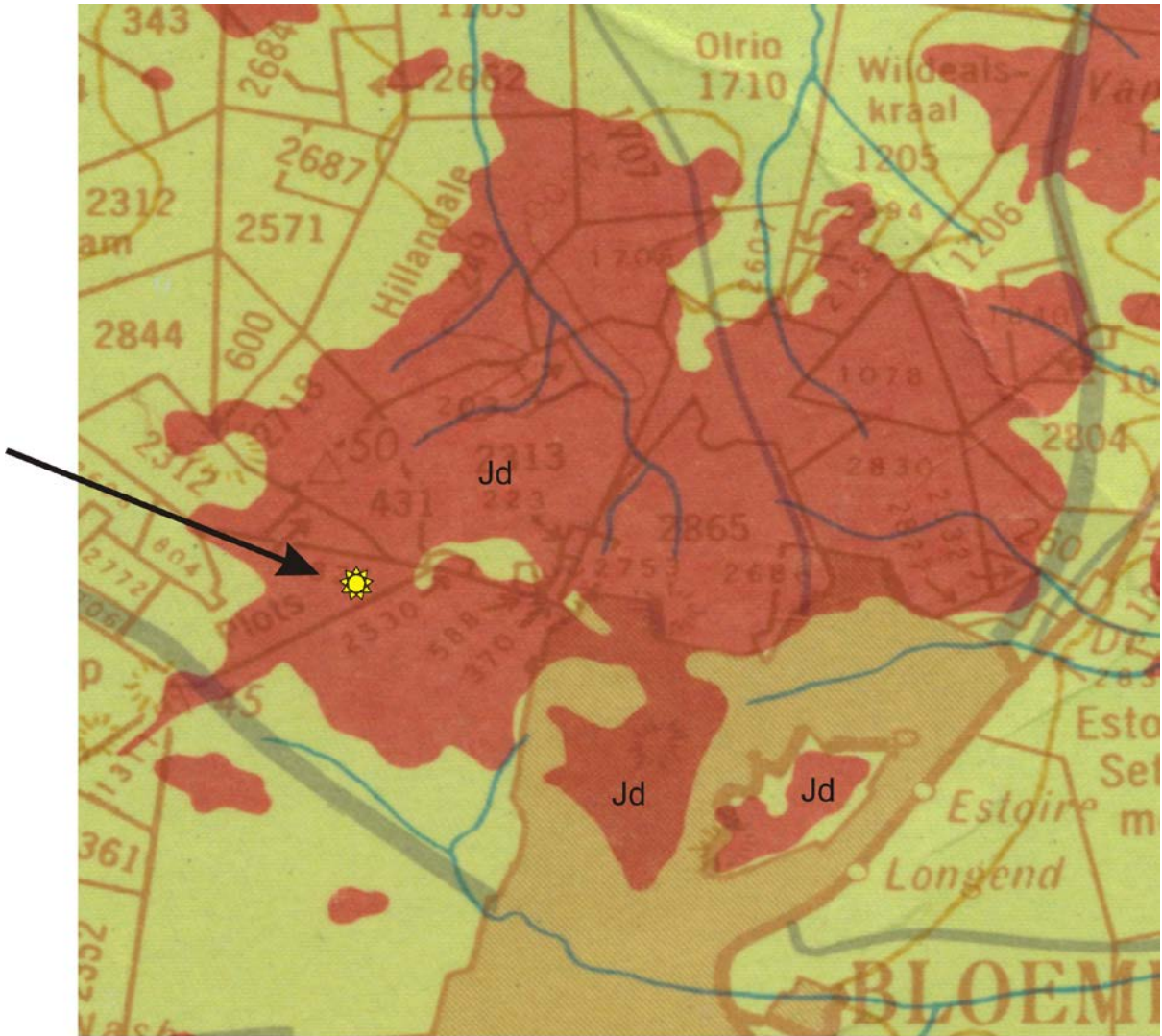
Figure 3. According to the 1:250 000 scale geological map 2926 Bloemfontein, the development footprint and surrounds are underlain by Jurassic igneous intrusions in the form of dolerite sills and dykes (red areas, marked Jd on map).
