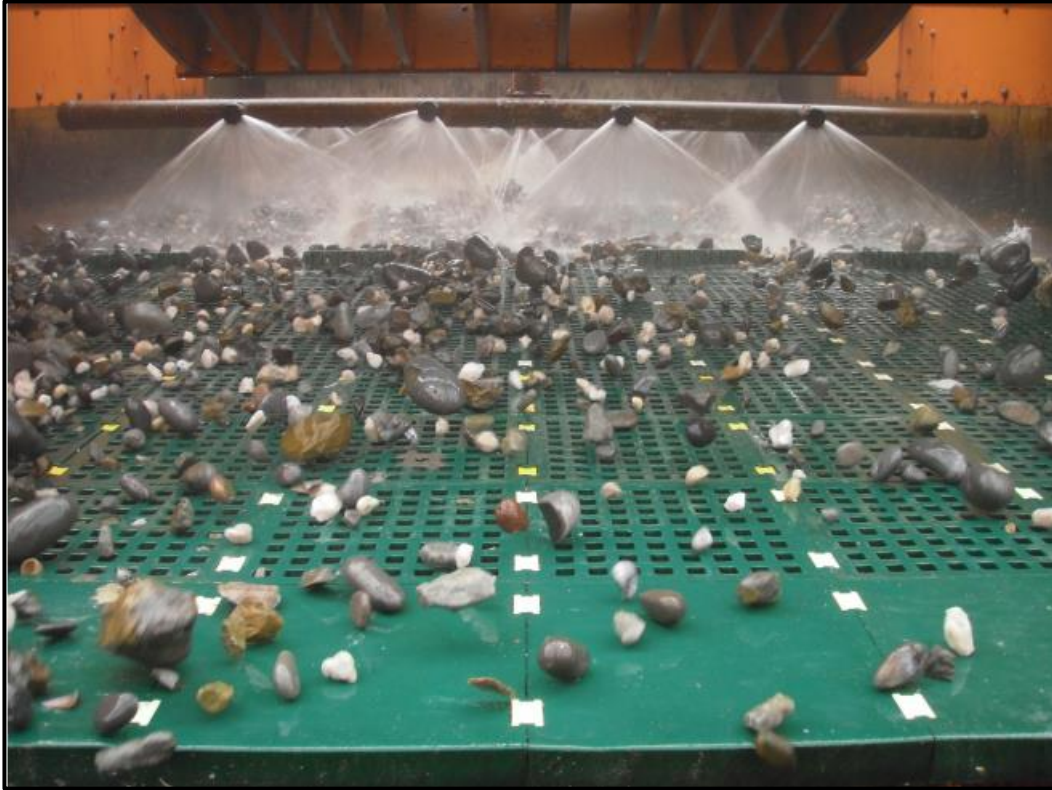
Figure 6. The gravel oversize screen on a typical diamond mining vessel where the geological personnel monitor the material being dredged and where fossil collection takes place.
