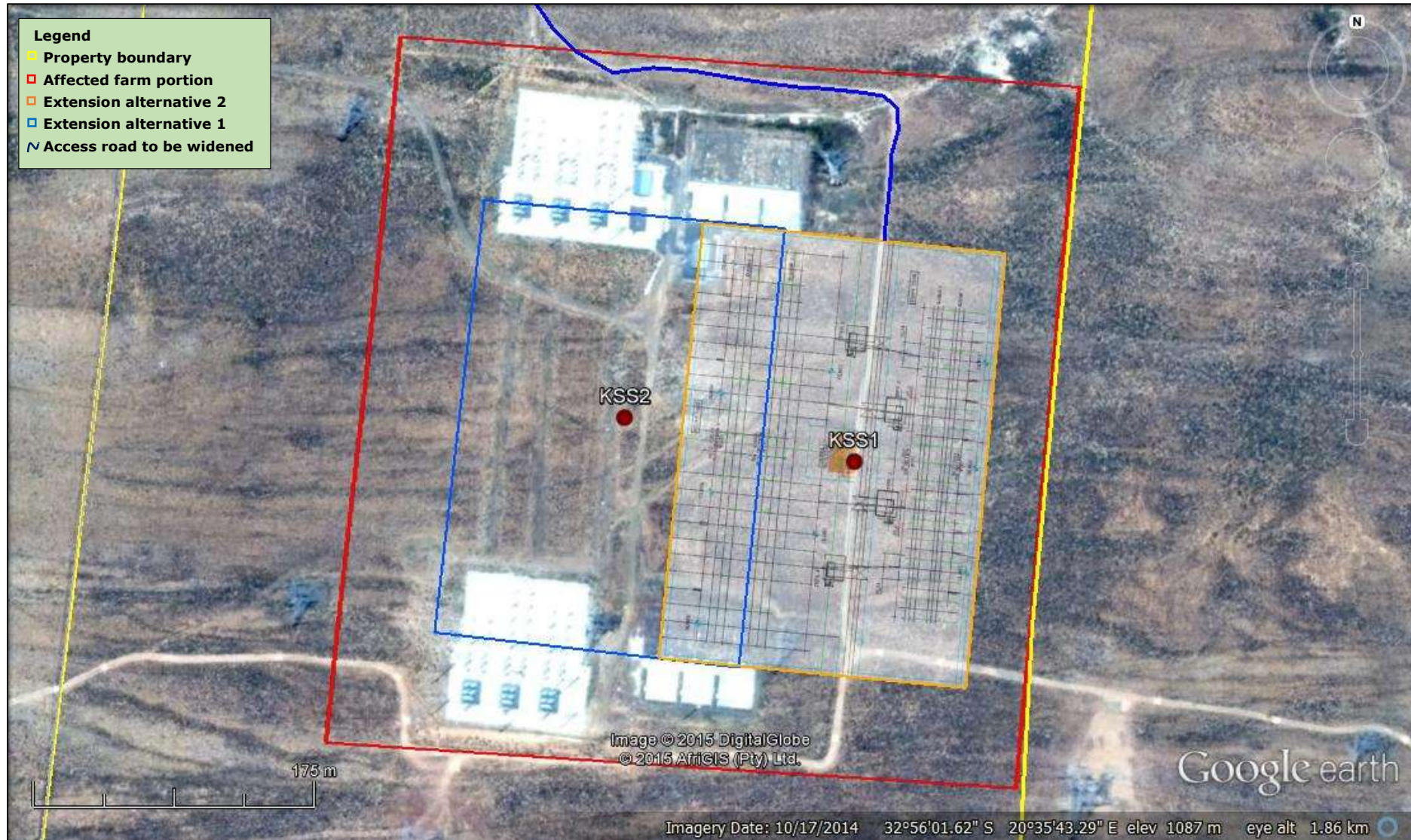
Figure 4. Close-up aerial view showing the location of the proposed extension of the existing Komsberg Substation (Alternative 1 and Alternative 2) and general GPS co-ordinates (KSS1 and KSS2).
