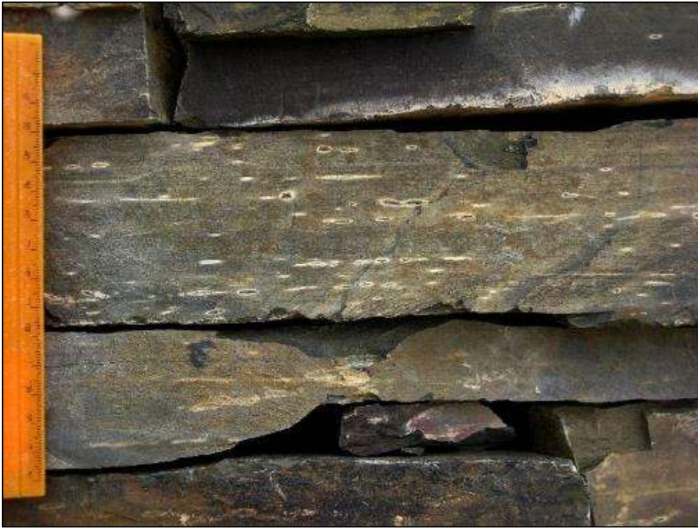
Fig. 23. Vertical sections through baked Tierberg Formation mudrocks used as building stones at Roodewerf, showing elliptical sections through burrow systems that are concentrated at specific horizons (Scale in cm).
