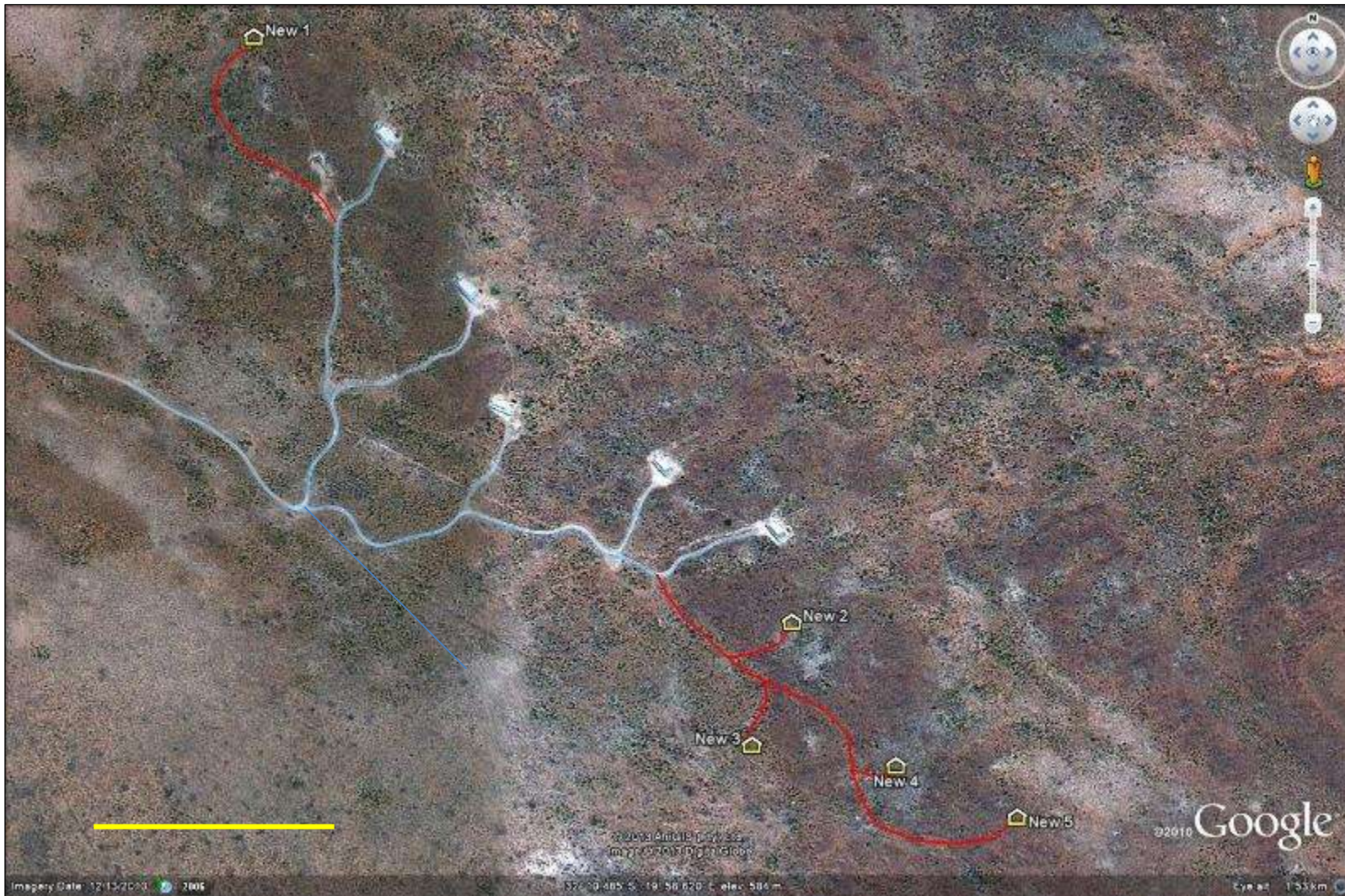
Fig. 2. Google earth© satellite image of the Elandsberg Rest Camp area showing the existing roads and buildings as well as the proposed five new accommodation units. Scale bar = c. 200 m. Image kindly provided by the Tanqua Karoo National Park.
