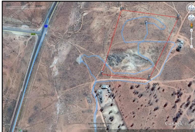
Figure 8: The borders of the extended borrow pit are shown in red and the tracks of the field survey in blue.
