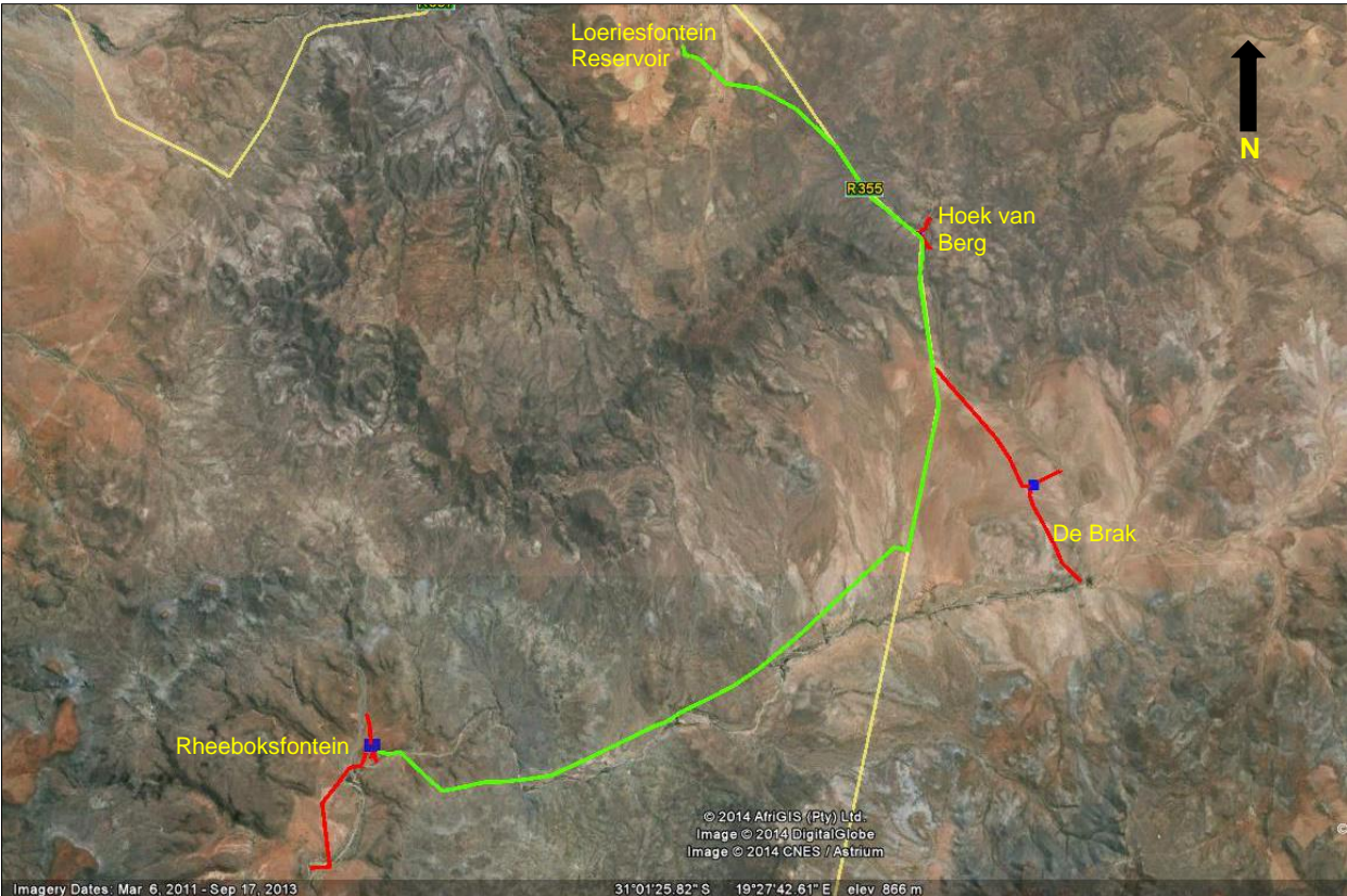
Figure 2. Google Aerial photograph indicating the proposed infrastructure for the Loeriesfontein Bulk Water Supply Pipeline and Reservoir. The main pipeline (rising main) is in green, while the feeder pipelines are in red. The blue polygons are the proposed new holding reservoirs, one of which is also planned at Hoek van Berg.
