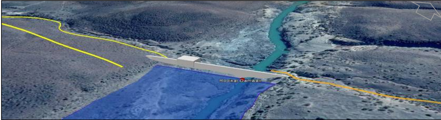
Figure 3: Modelled impression of the Rooikat Hydroelectric Power Site and dam wall (weir), with the power line and South Access Road alignments (left – yellow lines) and the North Access Road (right – orange line)
