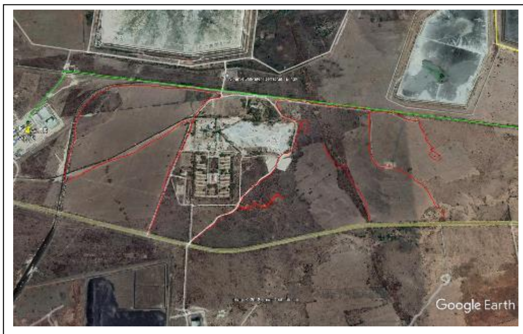
Figure 2- The GPS track log which the surveyor followed (red line) when covering the project area (above).
