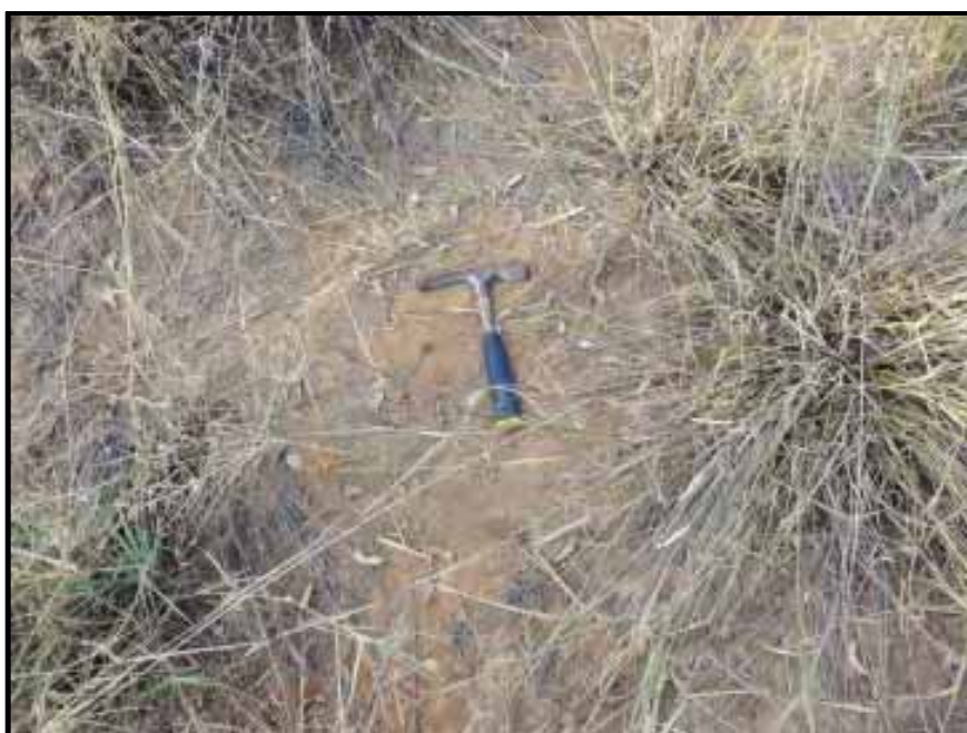
Figure 15: Unconsolidated orange-red, coarse-grained sands of the Cenozoic regolith (waypoint Lep 26, see Figure 3). The grass evident in the image is a species of Eragrostus that indicate that the regolith is at least 3.5 m thick in the area (information courtesy of Mr Alan Bosman pers comm. ).
