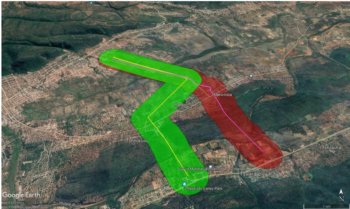
Figure 2: Google Earth Map of the proposed Tshilamba 132 kV powerline routes and 300m corridors.
