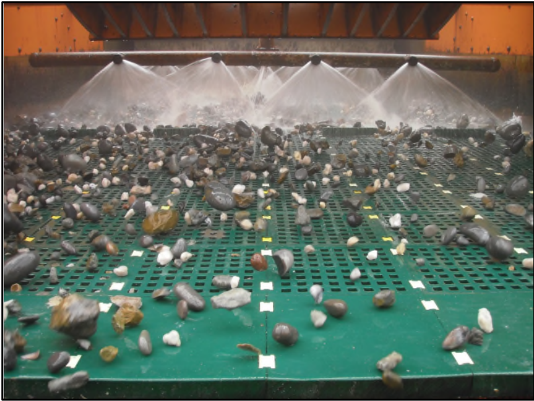
Figure 6. The gravel oversize screen on a typical diamond sampling vessel where the geological personnel monitor the material being dredged and where fossil collection takes place.
