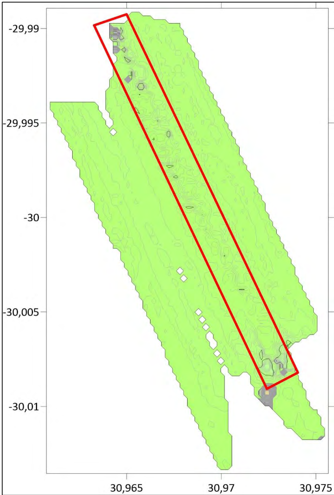
Figure 8: Magnetometer Survey Mosaic with Pipeline marked
