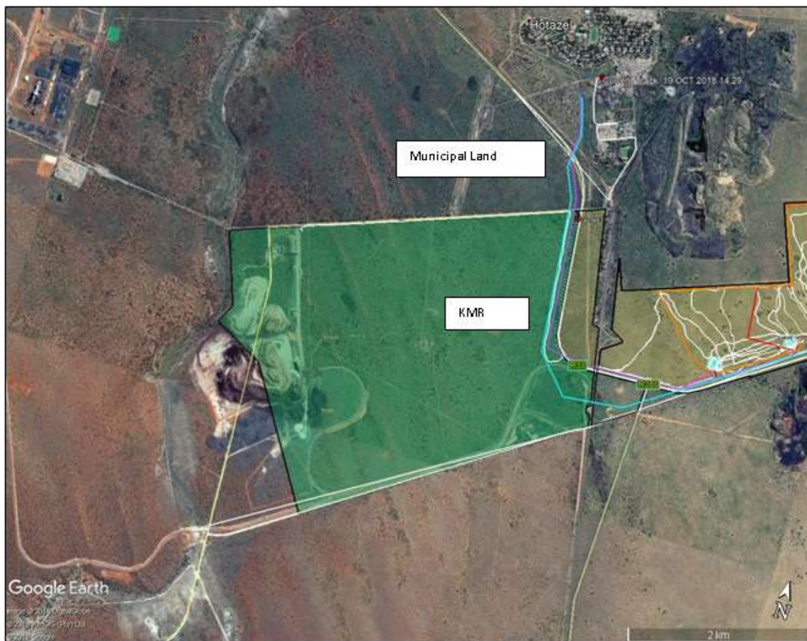
Figure 17: The route of the proposed 132 kV powerline, from York A 279, across the railway line and R31, through the property of KMR and Municipal land, connecting with the Hotazel substation, a distance of 6km in total. Our tracks are shown in white.
