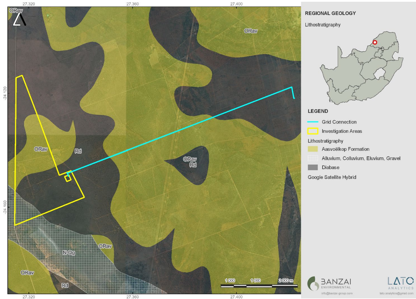
Figure 5: Updated Geology (Council of Geosciences, Pretoria) of the proposed Mirarch Solar PV Project near Thabazimbi, Limpopo Province indicates that a portion of the development is underlain by the alluvium, colluvium, eluvium and gravel while the rest is underlain by diabase and the Aasvoëlkop Formation of the Waterberg Group.
