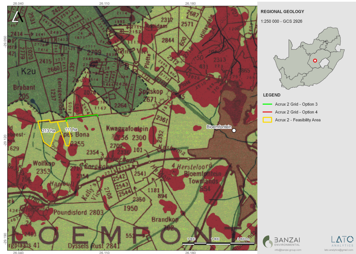
Figure 7. Extract of the 1:250 000 Bloemfontein 2926 Geological map (1966) (Council of Geoscience, Pretoria) indicating the geology of the Acrux Solar PV Project Two SPP and associated grid infrastructure near Bloemfontein in the Free State. The development is underlain by the Lower Stage (K31) of the Beaufort Group, Karoo System while a small area is underlain by dolerite.
