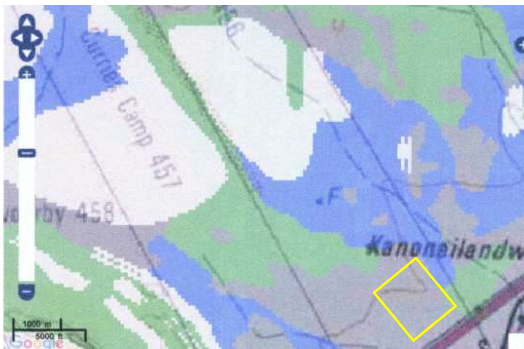
Figure 4: SAHRIS palaeosensitivity map for the site of the proposed Bushmanland PV is shown within the yellow rectangle. Background colours indicate the following degrees of sensitivity: red = very highly sensitive; orange/yellow = high; green = moderate; blue = low; grey = insignificant/zero.
