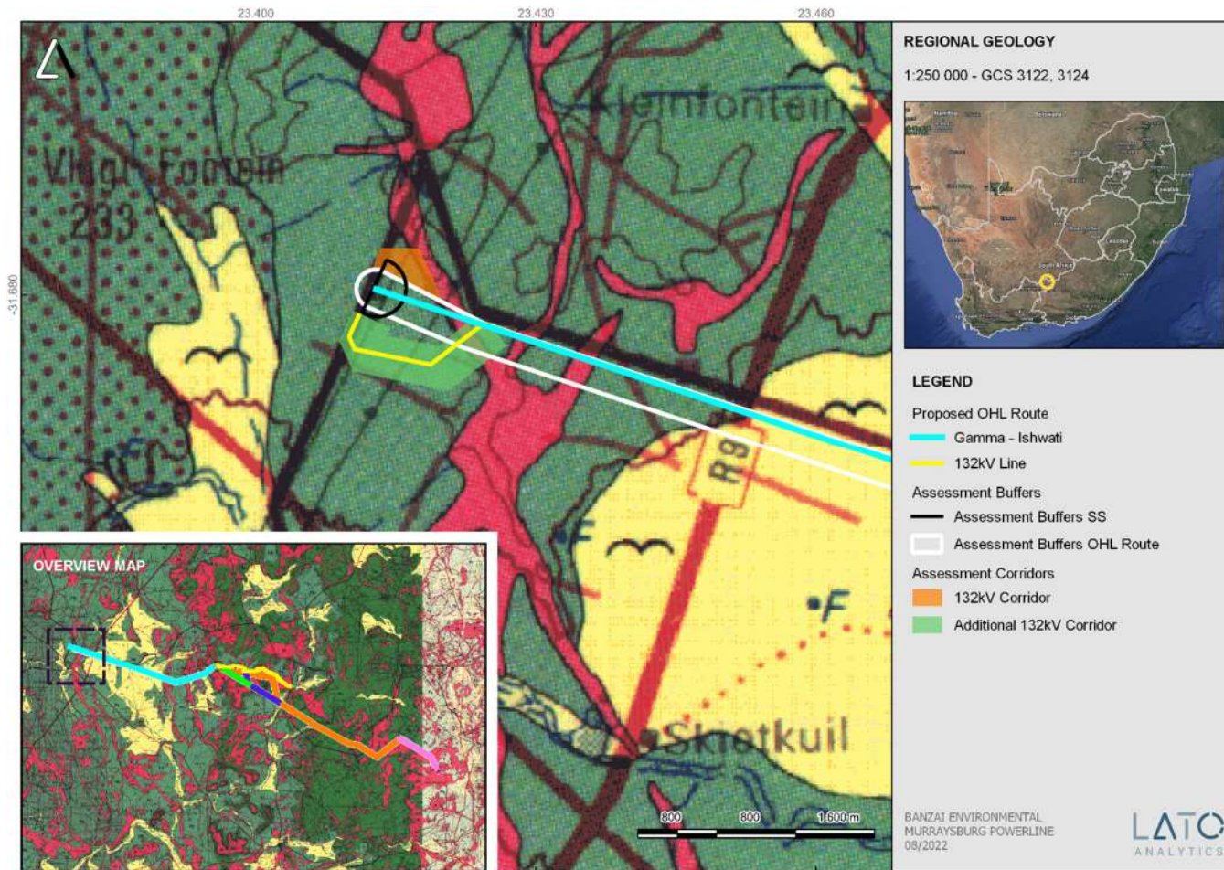
Figure 3: Extract of the 1:250 000 Victoria West 3122 (1989) Geological map (Council of Geoscience, Pretoria) indicating the Gamma substation and western margin of the proposed development underlain by Jurassic dolerite (red, Jd), Quaternary superficial deposits (yellow, single bird figure), and Teekloof (Pto / Pth, dark green) Formation of the Adelaide Subgroup
